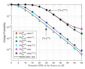
Fig. 5: Comparison study on the outage probability results of CR-NOMA using SA and TA schemes with EH.
