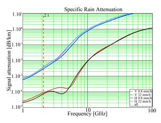
Fig. 2: Graph of the signal attenuation at 0.8 (annual average density) and 32 mm·h<sup>-1</sup> (relative rain rate for 0.01 %).
