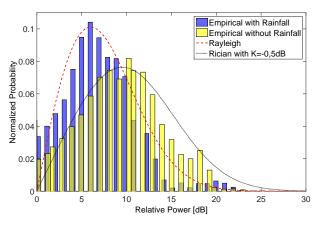
Fig. 4: Fitting the probability density functions to the empirical data for NodeB with PSC 444.
