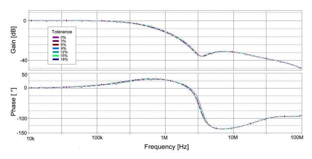
Fig. 7: Amplitude and phase frequency response of second order low-pass filter.
