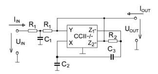
$\begin{tabular}{ll} \bf Fig.~5:~Second~order~low-pass~filter~with~synthetic~immittance\\ element. \end{tabular}$
