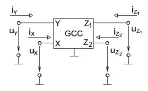
Fig. 1: Schematic symbol of four-port general current conveyor.
