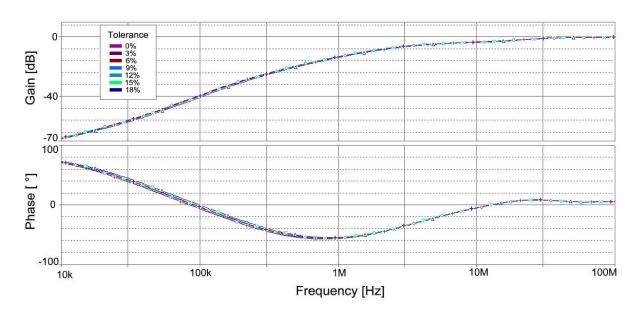
$\textbf{Fig. 8:} \ \, \textbf{Amplitude and phase frequency response of second order high-pass filter}.$
