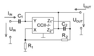
Fig. 6: Second order high-pass filter with synthetic immittance
