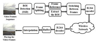
Fig. 1: The proposed streaming technique.
