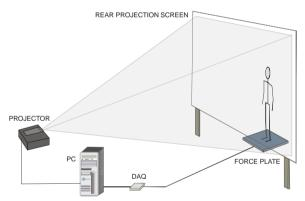
Fig. 2: Components of the proposed measurement system.
