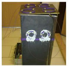
Fig. 21: The crystallizer model with covered upper part and NTC sensor of digital thermometer TESTO 720.
