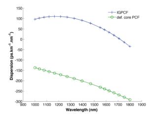
Fig. 2: Comparison of IGPCF with a solid core and investigated PCF with modified core geometry.
