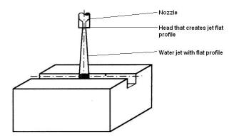
Fig. 1: The application of high-velocity water jet to a concrete surface, groove cutting.
