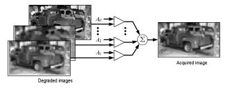
Fig. 8: Model of the image fusion.
