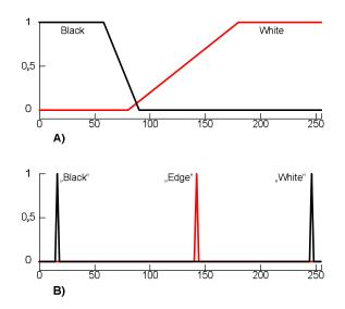
**Fig. 2:** Membership function of the input image (A) and output image (B).
