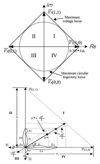
vector PWM modulation (SVM) output voltage for twophase inverter according to [10] is shown in Fig. 5.
