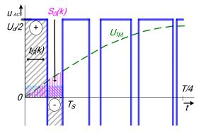
**Fig. 9:** PWM with even multiply of  $f_1$ .
