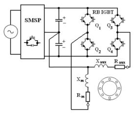
Fig. 14: Circuit diagram of investigated of two-phase induction machine.
