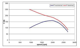
Fig. 17: Waveforms of electrical power of DC/AC/AC converter and mechanical power from 2-phase ASM motor.
