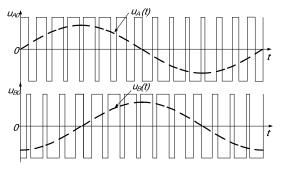
Fig. 7: Output orthogonal voltages of the half-bridge matrix converter system with bipolar PWM.
