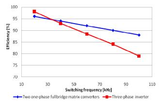
Fig. 10: Efficiencies of investigated inverter topologies depending up switching frequency. With RL load [14].
