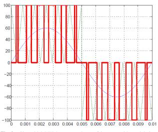
Fig. 3: Sinusoidal PWM output voltage of inverter with modulation index:  $m_a = 0.6$  and  $m_f = 12$ .
