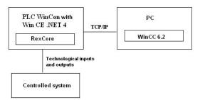
Fig. 6: Control system block scheme.
