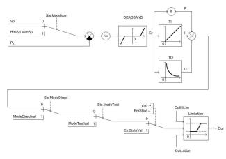
**Fig. 4:** The simplified function block scheme of the implemented PID regulator.
