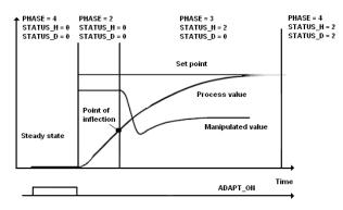
Fig. 1: The step response method by PID Self Tuner [3].
