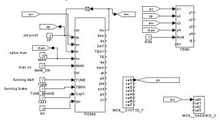
Fig. 7: Simulation scheme with PIDMA function block.
