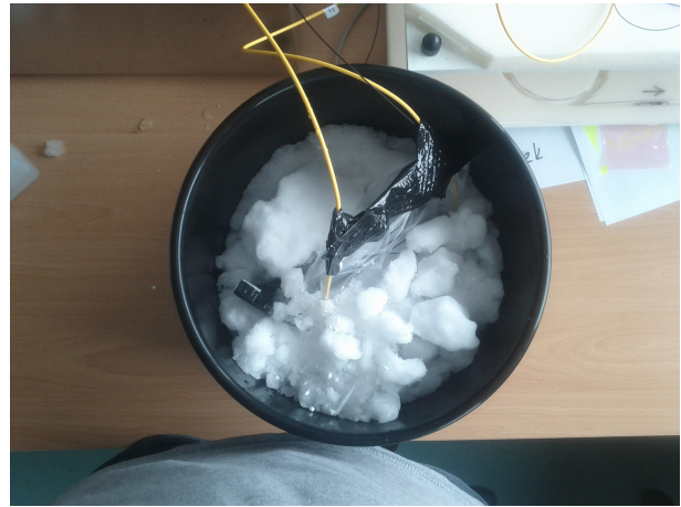
Fig. 6: Testing erbium doped fiber IsoGain I-6 at 1 °C temperature.
