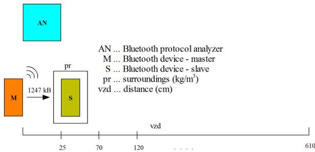
Fig. 3: Measuring workplace.
