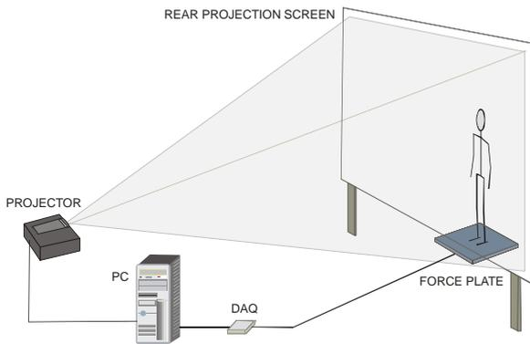
Fig. 2: Components of the proposed measurement system.
