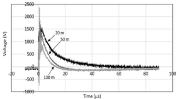
Fig. 3: Measured voltage traces at various distances from a single rod electrode, installed at site 2, injected at 100 kV.
