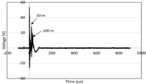
Fig. 2: Measured voltage traces at various distances from a single rod electrode, installed at site 1, injected at 100 kV.
