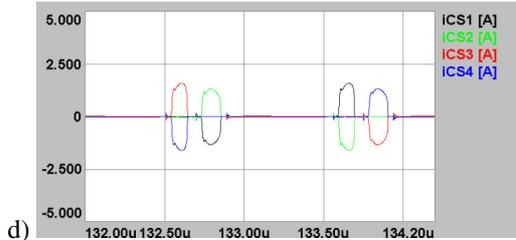
Fig.11. Current and voltage waveforms during transistor switching;  $\gamma=0$ ,  $\beta=0.18$ ,  $f=475\text{kHz}$ ,  $R=60\Omega$
