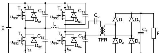
Fig. 1. ZVS bridge MRC
