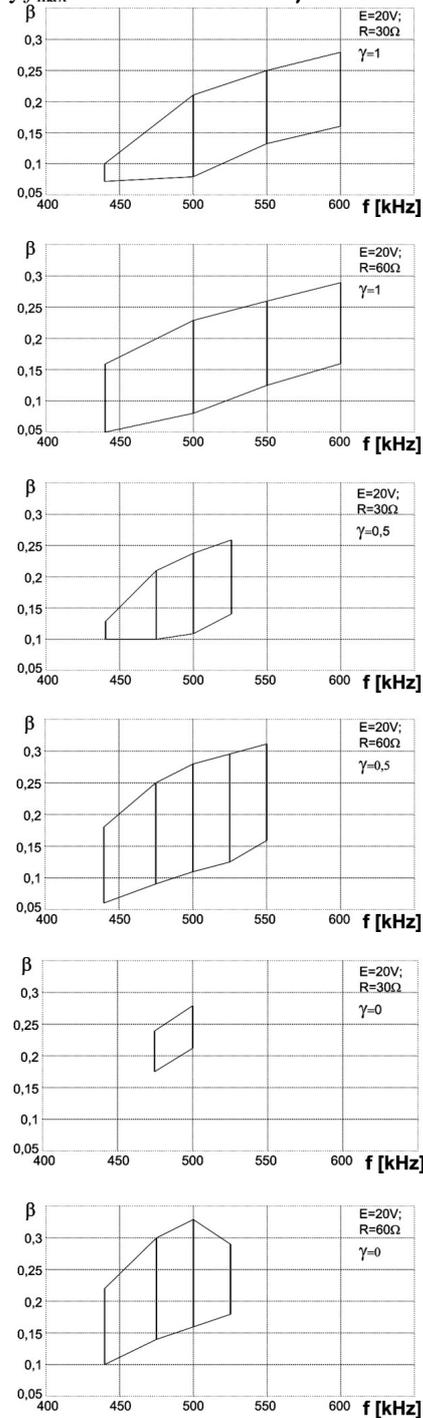
Fig.6. ZVS operation area of the bridge converter for a)  $R=30\Omega,$  b)  $R=60\Omega$
