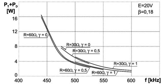
Fig.12. Total power losses in semiconductor elements of the ZVS bridge MRC
