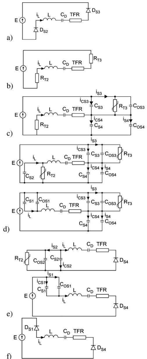
Fig.4. Resonant circuits of the ZVS bridge MRC a) for  $(t_1 \leq t \leq t_2)$ , b) for  $(t_2 \leq t \leq t_4)$ , c) for  $(t_4 \leq t \leq t_6)$ , d) for  $(t_6 \leq t \leq t_7)$ , e) for  $(t_7 \leq t \leq t_9)$ , f)  $(t_9 \leq t \leq t_{10})$
