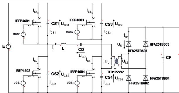
Fig.5. Simulation model of ZVS bridge MRC
