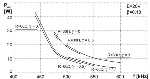
Fig.14. Output power  $P_{out}$  of the ZVS bridge MRC
