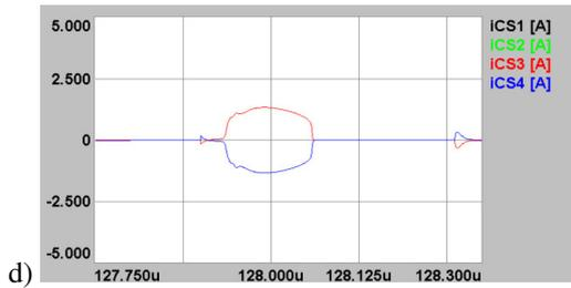
Fig.10. Current and voltage waveforms during transistor switching;  $\gamma=1$ ,  $\beta=0.18$ ,  $f=500\text{kHz}$ ,  $R=60\Omega$
