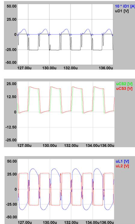
Fig.7. Current and voltage waveforms in ZVS bridge MRC,  $R=60\Omega$ ,  $f=500\text{kHz}$ ,  $\beta=0.18$ ,  $\gamma=0.5$
