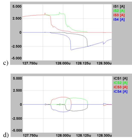
Fig. 9. Current and voltage waveforms during transistor switching, at;  $\gamma=0,5, \beta=0,18, f=500kHz, R=60\Omega$  a) control signals, b) transistor voltages, c) transistor currents, d) snubber capacitors currents
