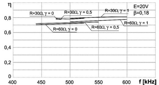
Fig.13. Efficiency  $\eta$  of the ZVS bridge MRC
