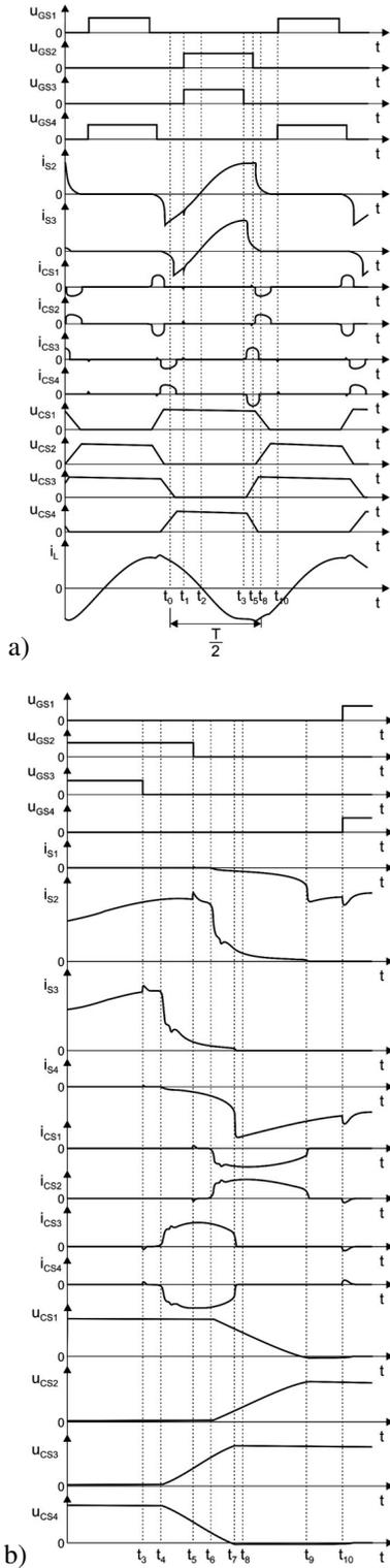
Fig.3. Current and voltage waveforms in the ZVS bridge MRC shown in Fig. 1, a) during a half of the operation cycle  $\Delta t=T/2$  b) at switching between legs of  $T_3$ ,  $T_2$  and  $T_4$
