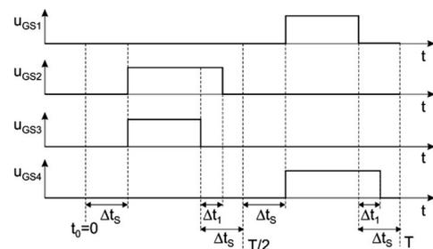
Fig. 2. Control signals algorithm of the ZVS bridge MRC shown in Figure 1
