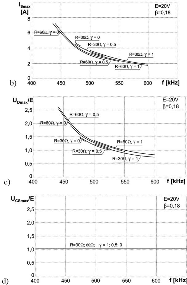
Fig. 8. Control characteristics of the ZVS bridge MRC, at  $R=30\Omega, R=60\Omega, \gamma=1, \gamma=0,5, \gamma=0$  a) conversion ratio  $M$ , b) maximum transistor current  $I_{Smax}$ , c) maximum diode voltage  $U_{Dmax}/E$ , d) maximum transistor voltage  $U_{CSmax}/E$
