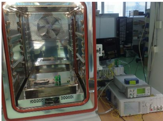
Fig. 2: The realized experimental set-up for temperature characterization of the IL and PDL spectral response of optical MUX/DEMUX.
