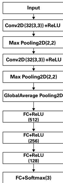
Fig. 2: Design of the proposed CNN structure.
