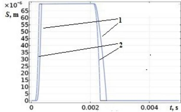
Fig. 4: Dependencies of the armature stroke (forward and reverse stroke for one cycle) for the basic design option (1) and the improved one (2).
