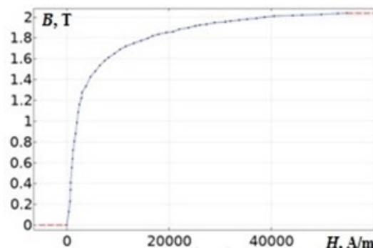
Fig. 3: Magnetization curve of the material of the 16MnCr5 brand.
