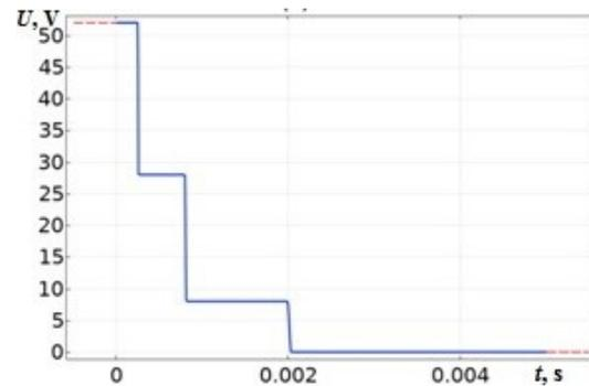
Fig. 2: The shape and values of the voltage on the winding as the function of time set by external source (microprocessor control).
