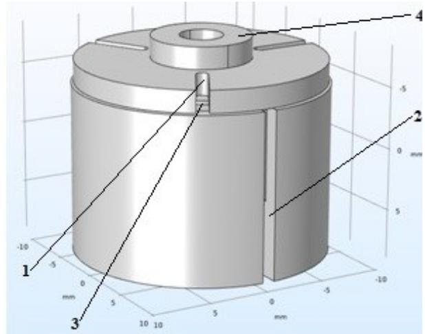
**Fig. 1:** 3D model of the electromagnet prepared in AutoCAD and imported to Comsol Multiphysics: 1 - the cutouts in the armature; 2 - the cuts in the housing; 3 - the winding placed inside the housing; 4 - the plane of attachment of the return spring.
