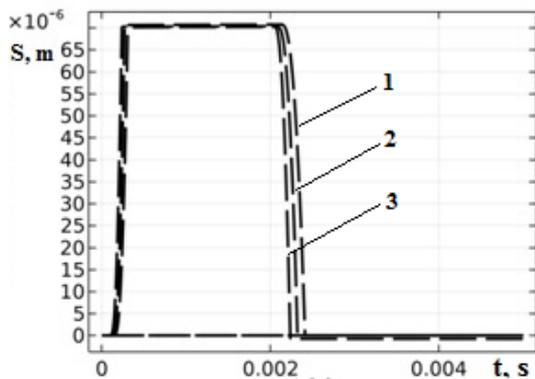
Fig. 10: Electromagnet actuation dynamics as a function of material resistivity:  $10 \cdot 10^{-8} \Omega \cdot m$  (1),  $18 \cdot 10^{-8} \Omega \cdot m$  (2),  $100 \cdot 10^{-8} \Omega \cdot m$  (3).
