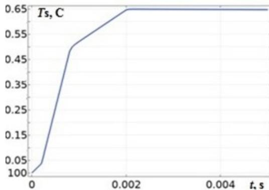
Fig. 12: Average temperature rise of the winding for one operating cycle of the electromagnet.
