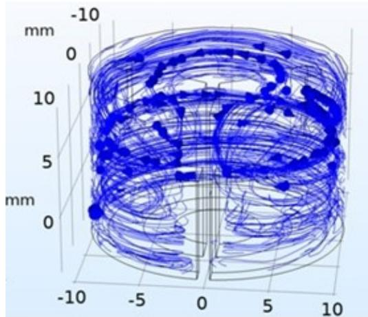
Fig. 9: The nature of eddy currents in the magnet housing at 0.13 ms.
