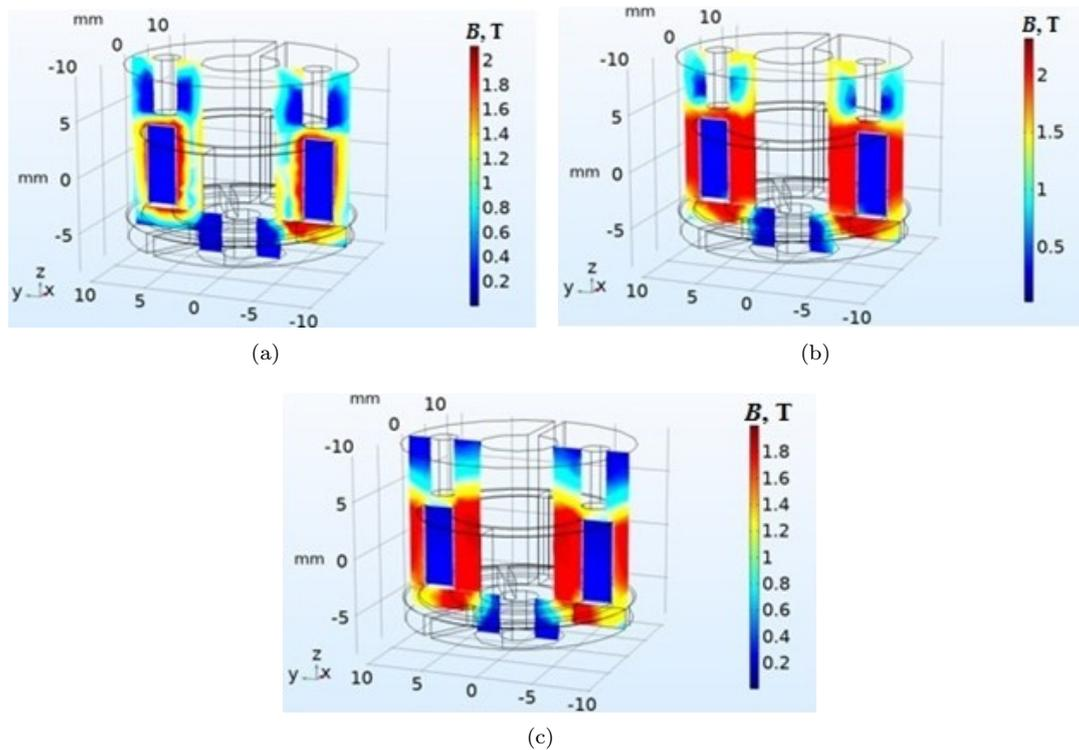
**Fig. 6:** The values of the modulus of the magnetic flux density in the housing of the electromagnet at different times, (a)  $t = 0.1$  ms, (b)  $t = 0.2$  ms, and (c)  $t = 0.3$  ms.
