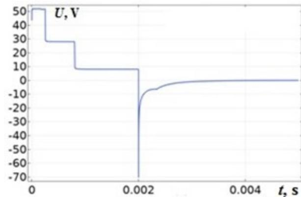
Fig. 5: Voltage on the electromagnet winding taking into account transients and the additional resistance in the winding circuit.
