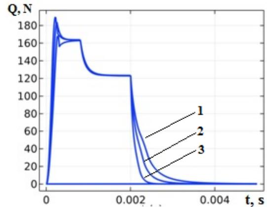
Fig. 11: Electromagnetic force as a function of material resistivity:  $10 \cdot 10^{-8} \Omega \cdot m$  (1),  $18 \cdot 10^{-8} \Omega \cdot m$  (2),  $100 \cdot 10^{-8} \Omega \cdot m$  (3).
