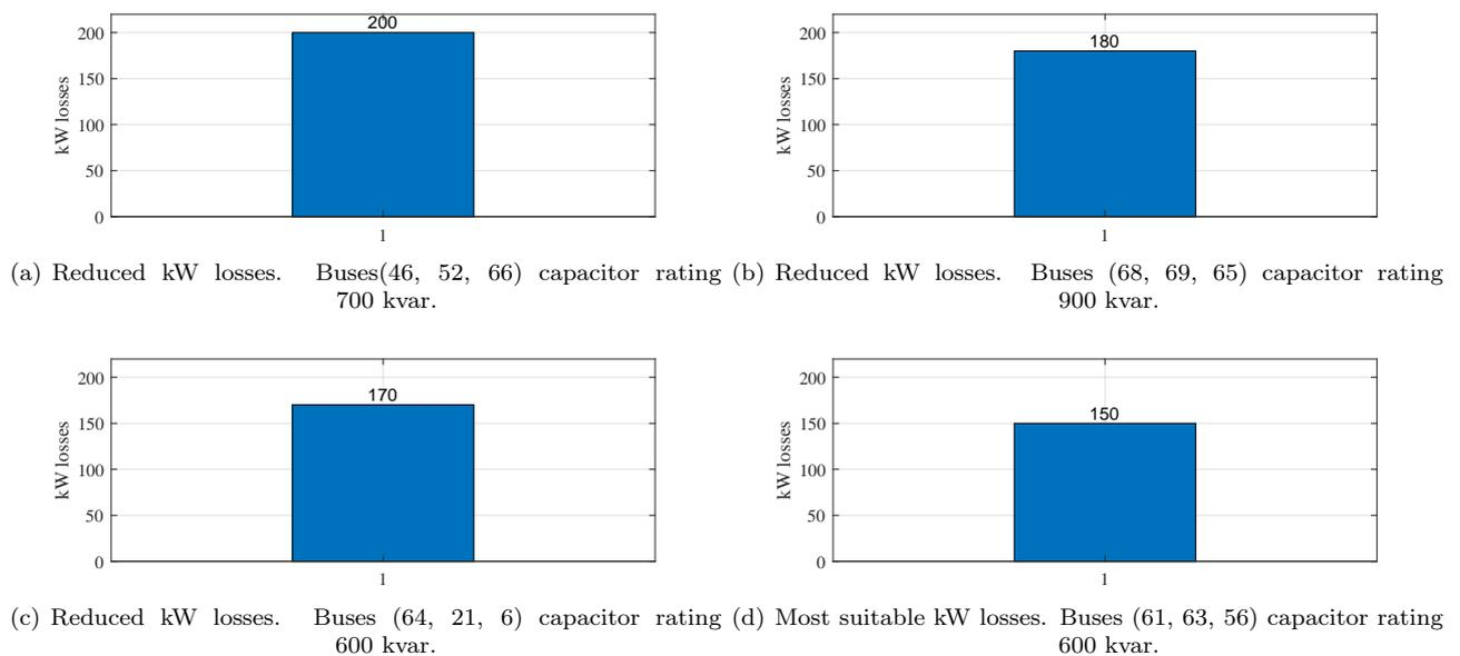
**Fig. 9:** Mitigation of power losses with different capacitor ratings for IEEE 69-bus system.
