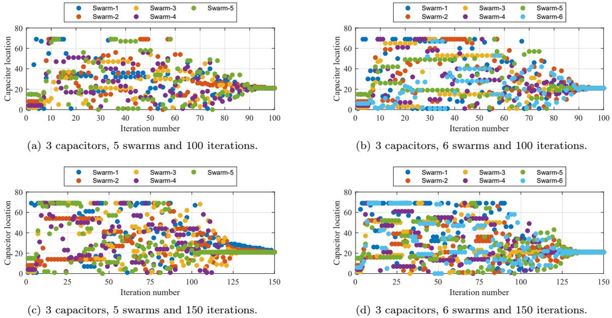
Fig. 19: Optimal capacitor location with identical capacitors having different swarms at 100 and 150 iterations.
