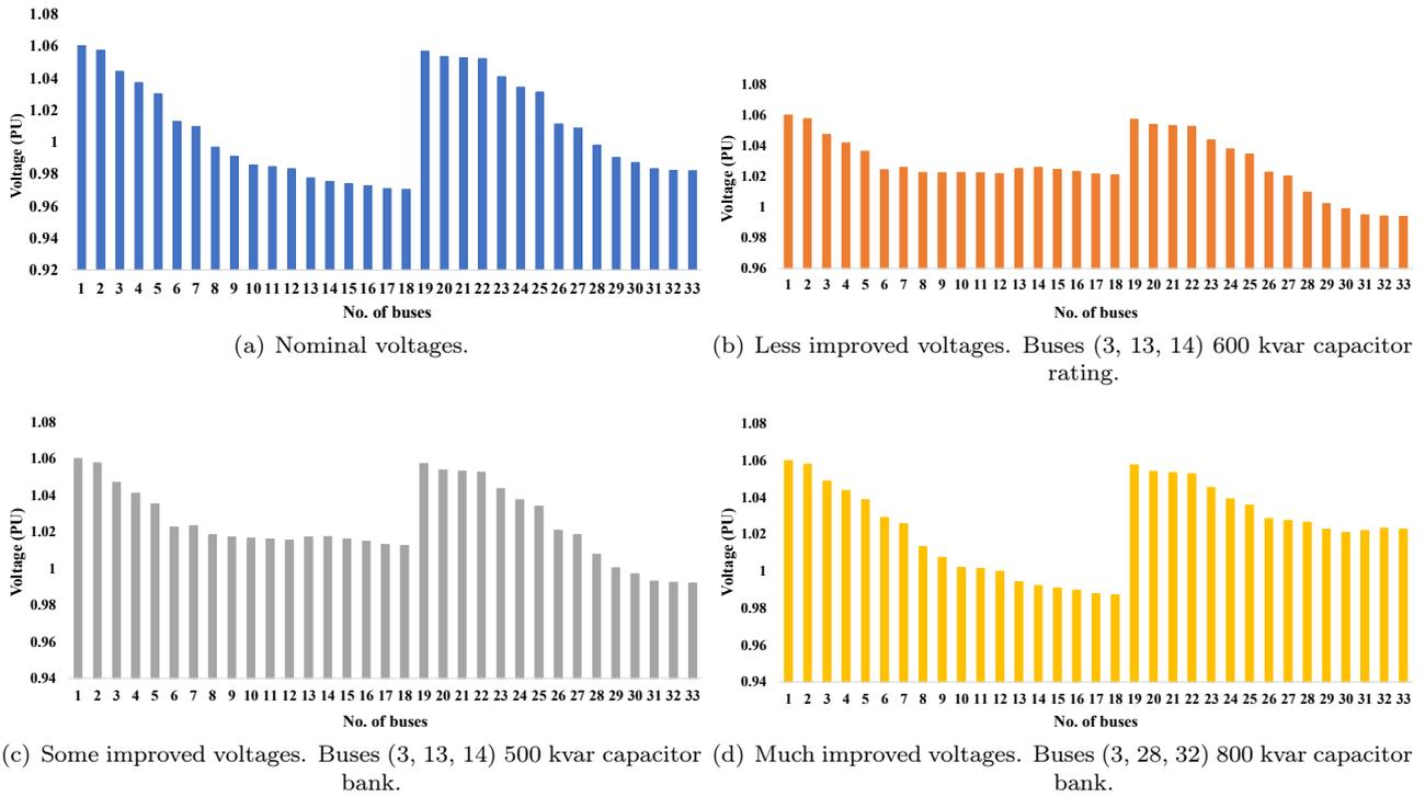
Fig. 4: PU voltages of IEEE 33-bus system with and without capacitor placement.
