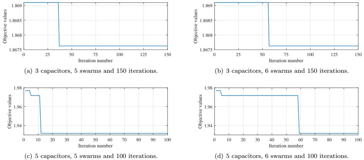
Fig. 12: Cost function with 3 and 5 capacitors having different swarms at various iterations.
