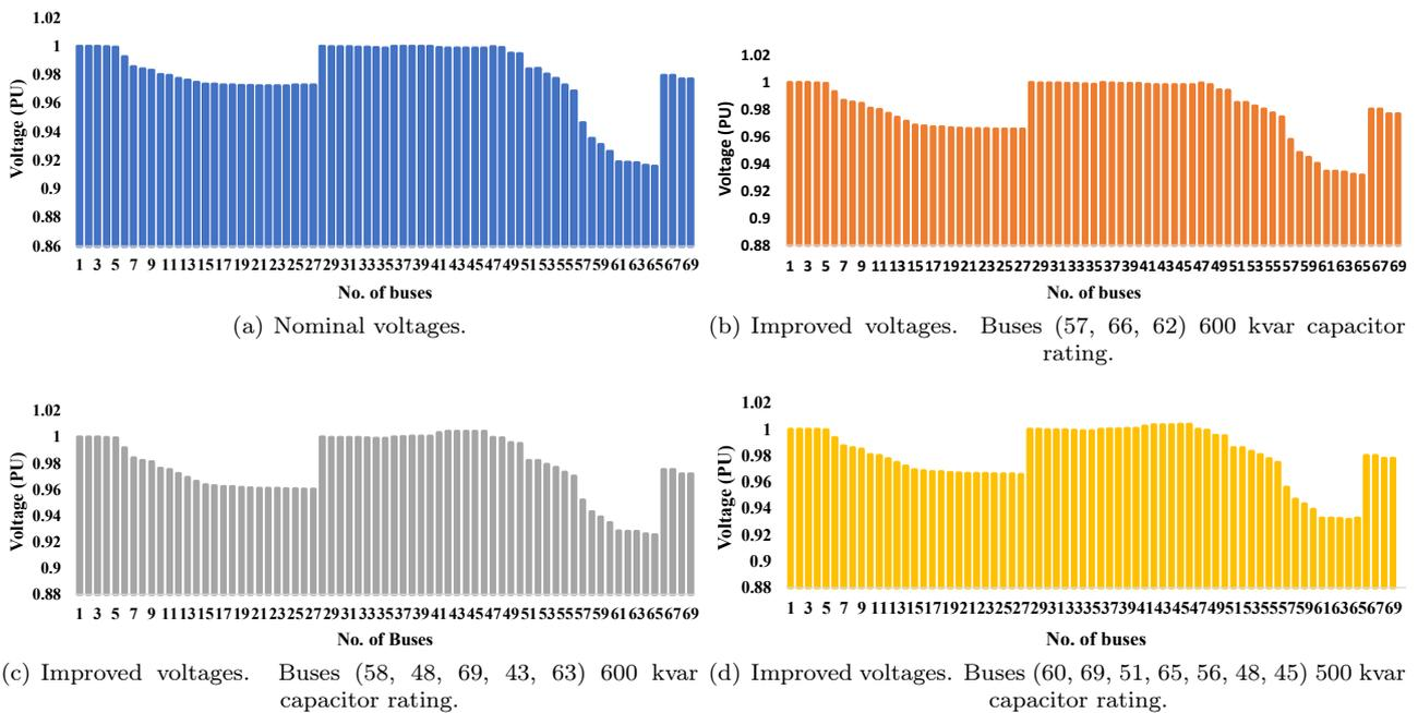
Fig. 5: PU voltages of IEEE 69-bus system with and without capacitor placement.
