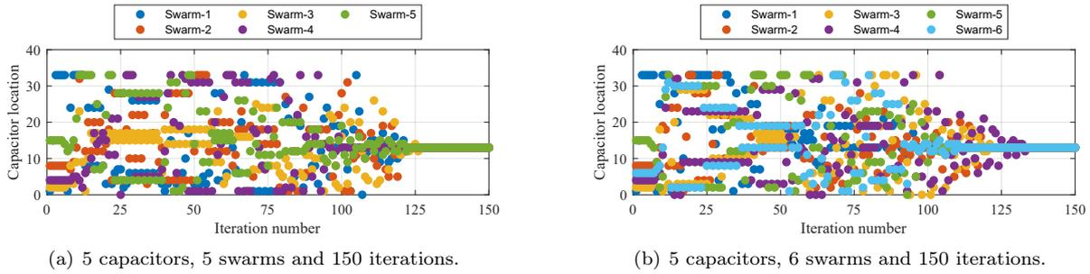
Fig. 16: Optimal capacitor location with identical capacitors having different swarms at 150 iterations.
