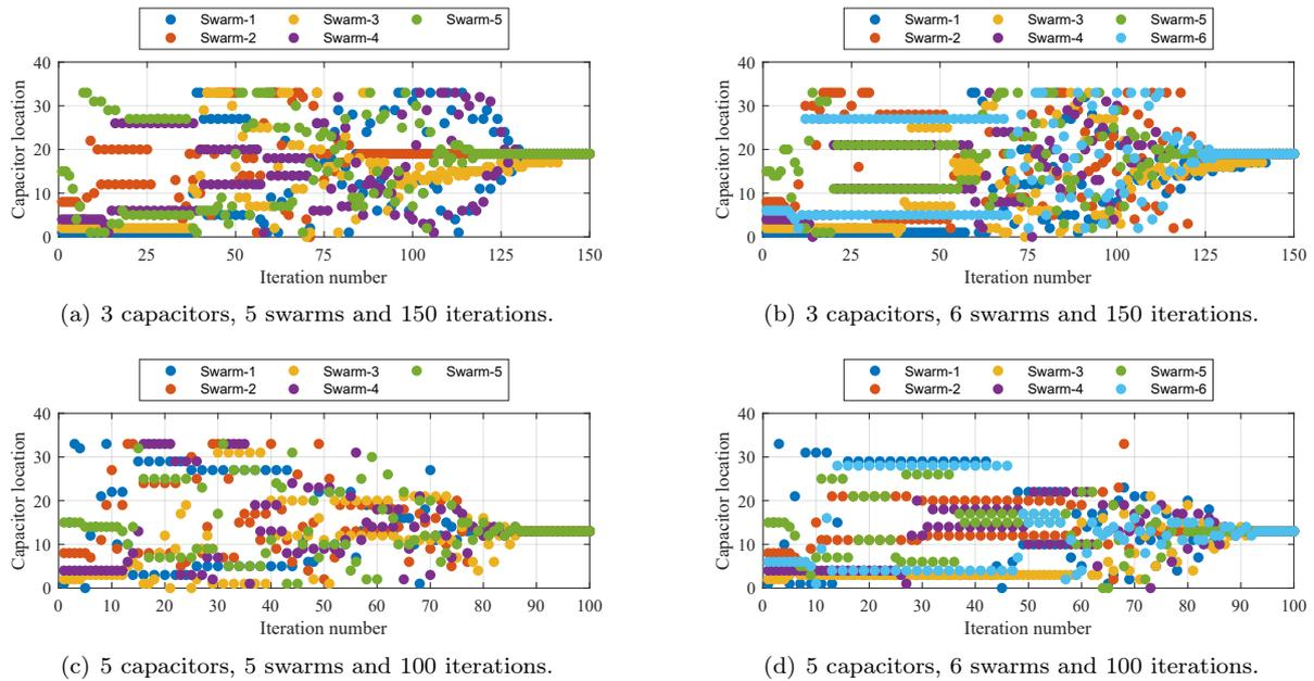
**Fig. 15:** Optimal capacitor location with identical capacitors having different swarms at 150 and 100 iterations.
