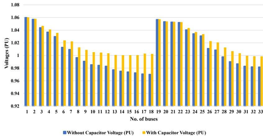
Fig. 6: Comparison of voltages with and without capacitor banks for IEEE 33-bus system.
