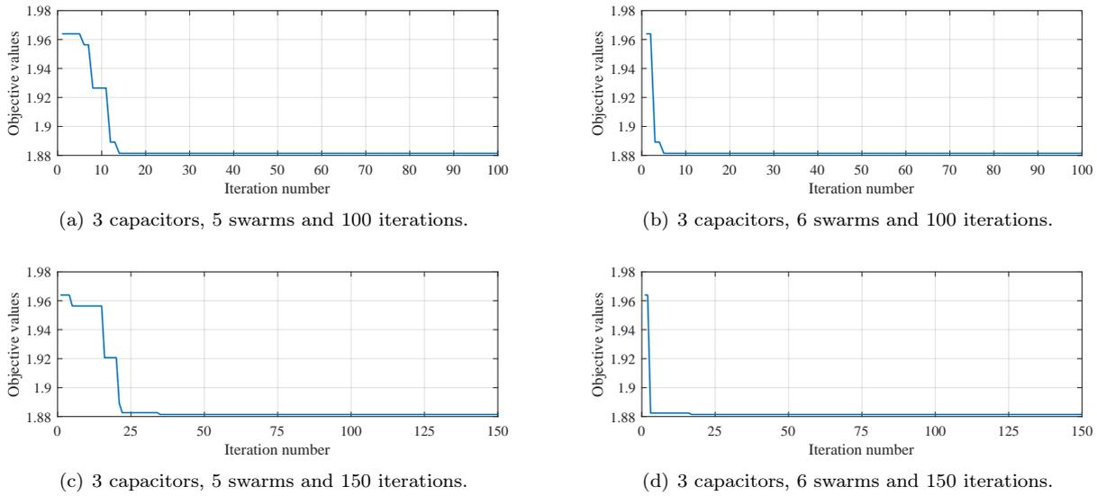
Fig. 17: Cost function with 3 and 5 capacitors having different swarms at various iterations.
