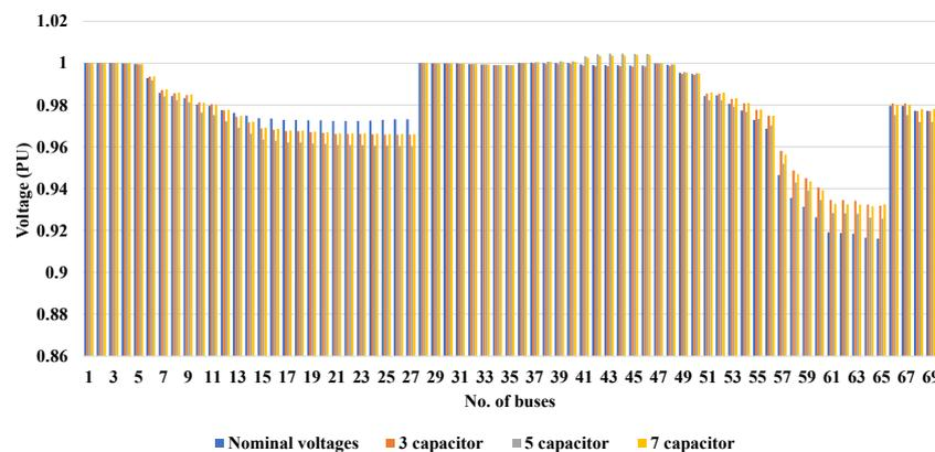
Fig. 7: Comparison of voltages with and without capacitor banks for IEEE 69-bus system.
