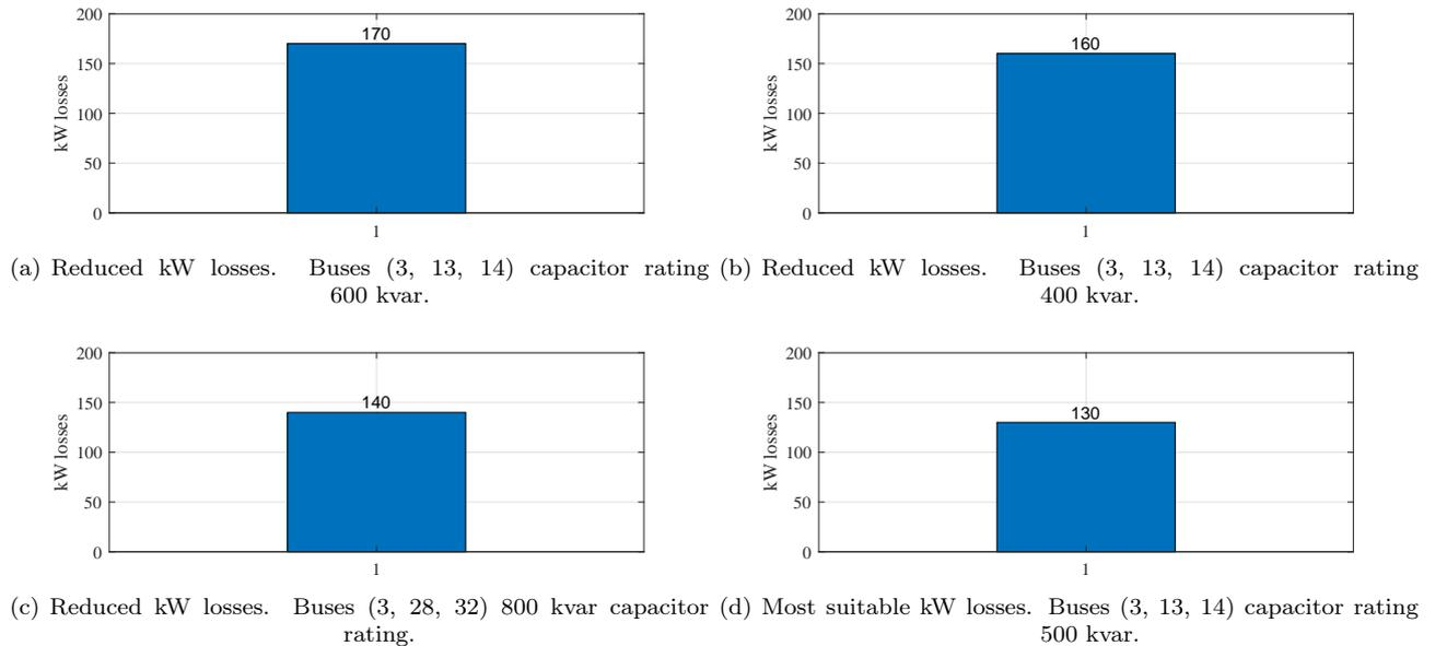
**Fig. 8:** Mitigation of power losses with different capacitor ratings for IEEE 33-bus system.
