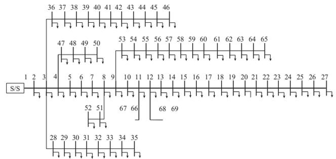
Fig. 2: SL diagram of IEEE 69-bus system [37].
