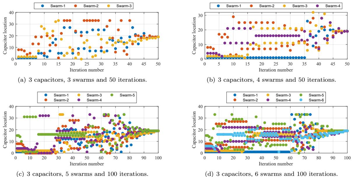
Fig. 14: Optimal capacitor location with identical capacitors having different swarms at 50 and 100 iterations.
