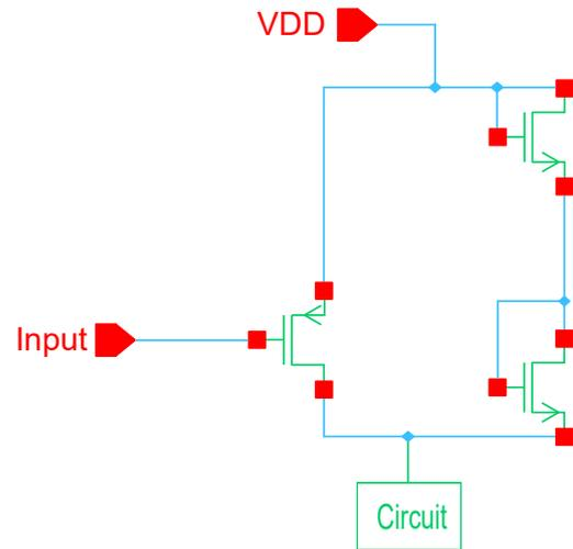
Fig. 6: Basic circuit illustrating AVLS.
