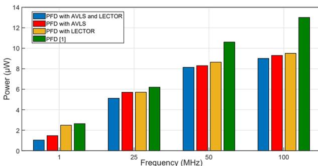
**Fig. 16:** Power of PFD architectures through range 1 to 100 MHz.
