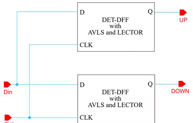
Fig. 14: PFD with AVLS and LECTOR techniques incorporated.
