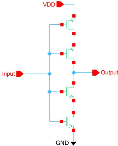
Fig. 8: Schematic of CMOS inverter with stack technique.
