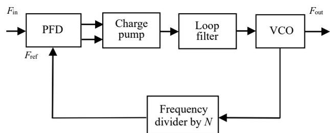
Fig. 1: Block representation of phase locked loop.
