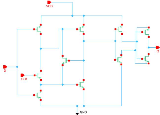
Fig. 9: Proposed circuit of DET-DFF with LECTOR technique.
