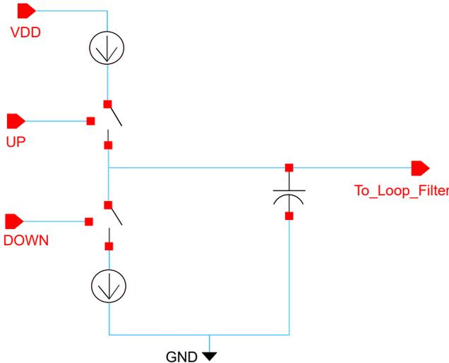
Fig. 2: Schematic of charge pump.
