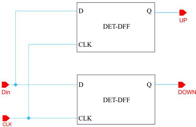
Fig. 4: Schematic of PFD realized using DET-DFF.
