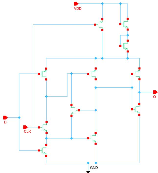
Fig. 10: Proposed circuit of DET-DFF with AVLS incorporated.
