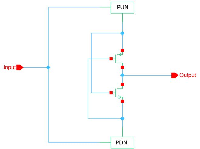
Fig. 5: A generic CMOS circuit with LECTOR technique.
