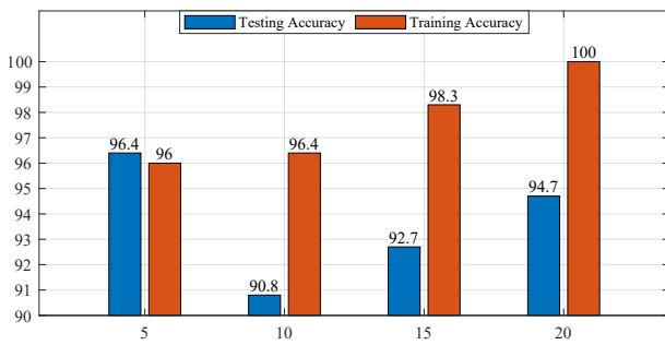
Fig. 3: Impact of window size on testing accuracy of DT model on distorted signal with all noise levels.
