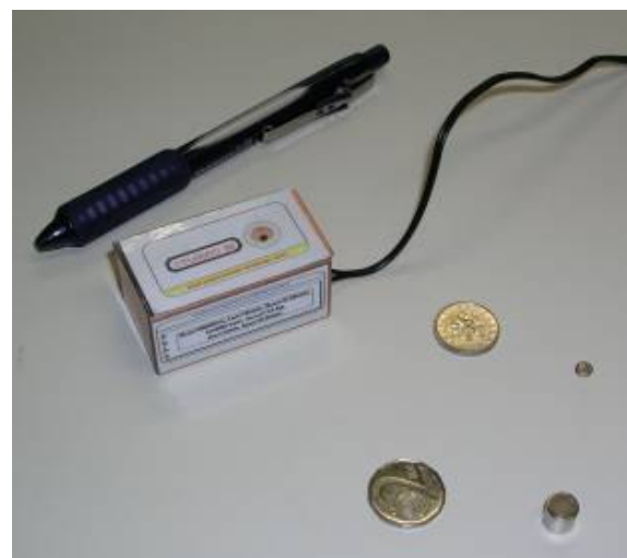
Fig.5. The first experimental prototype of vibrational mini-generator
