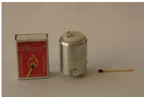
Fig.6. The second experimental prototype of vibrational mini-generator
