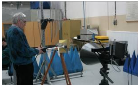
Fig.8. Calibration of calorimetric sensor
