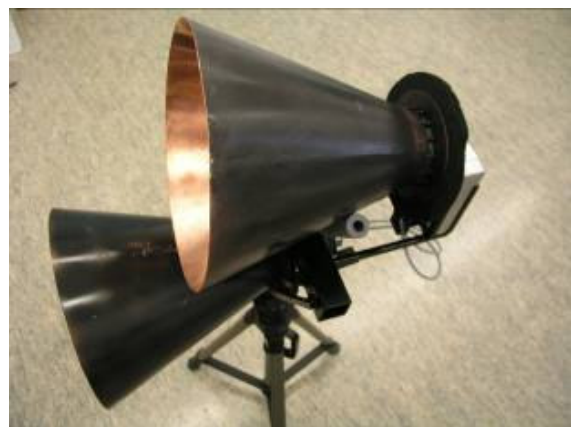
Fig.3. Realization of optimized combined calorimetric sensor
