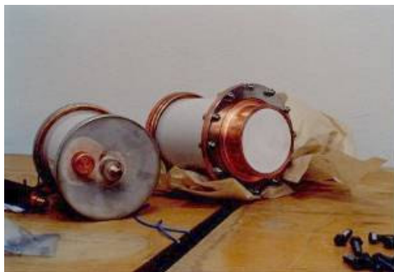
Fig. 5 Experimental construction of vircator, P_{\max} = 250 MW
