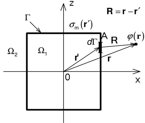
Fig. 4 Replacement of magnetization effect by surface magnetic charge at the area boundaries
