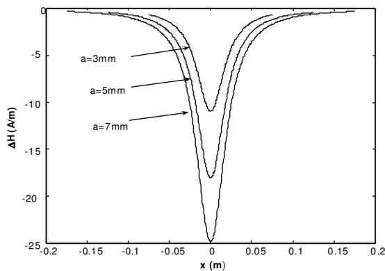
Fig. 8 Intensity of reaction magnetic field simulated by Matlab using collocation method
