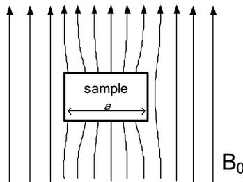
Fig 1. Magnetic flux density field deformation due to paramagnetic specimen
