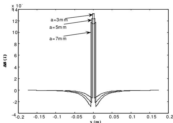
Fig. 9 Flux density of reaction magnetic field simulated by Matlab using collocation method
