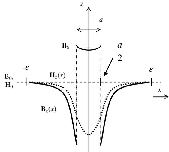
Fig 2. Ideal shape of magnetic intensity and flux density in paramagnetic specimen and its vicinity
