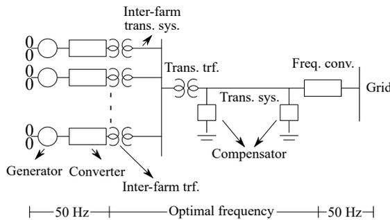
Fig. 1: Structure of electrical system for offshore wind power plant.
