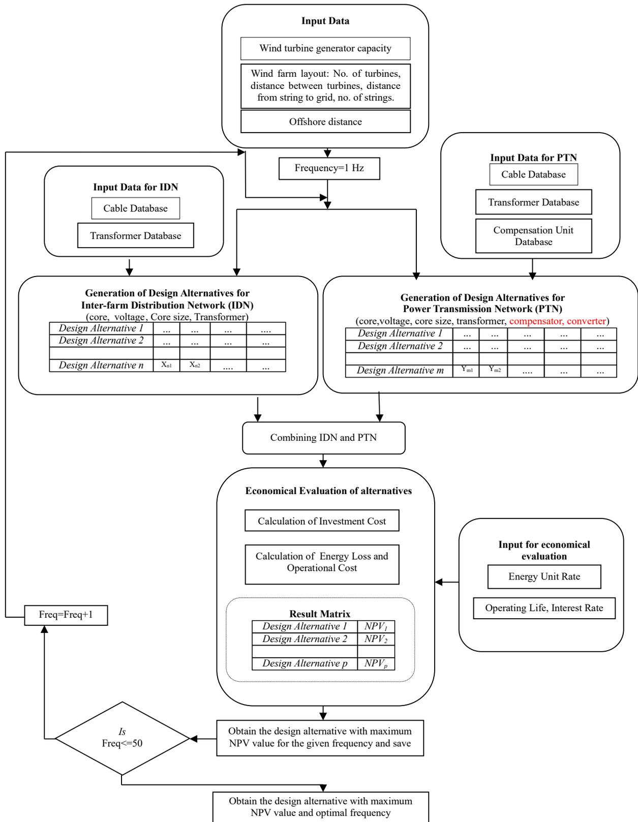
Fig. 2: Flow diagram for the design of ES.
