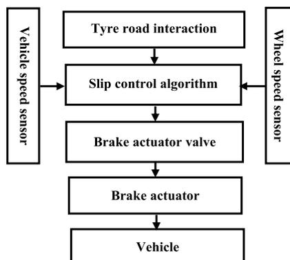
Fig. 1: Description of slip control in ABS.
