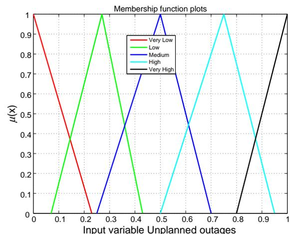
Fig. 1: Membership function plot for the input variable Unplanned outages.
