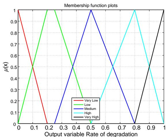
Fig. 5: Membership function Rate of Degradation used in Criteria 2.
