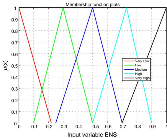
Fig. 2: Membership function plot for the input variable ENS.
