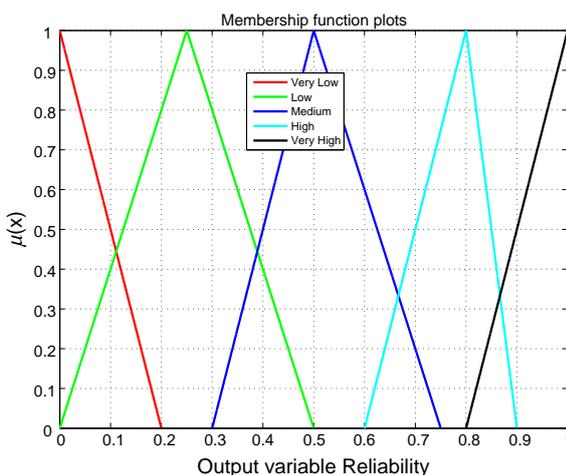
Fig. 3: Membership function plot for the output variable Reliability.
