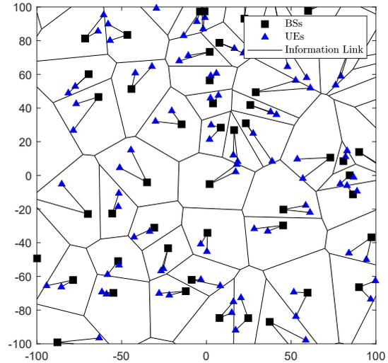
Fig. 1: A realization of the single-tier downlink NOMA with dense deployment of BSs.
