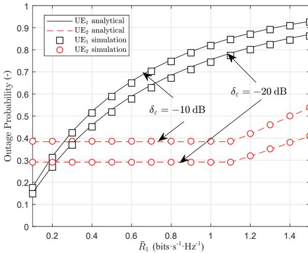
**Fig. 2:** Outage probability at each UE<sub>*i*</sub> with  $N = 2$ ,  $\bar{R}_2 = 0.2 \text{ bits}\cdot\text{s}^{-1}\cdot\text{Hz}^{-1}$  and  $P_1 = 0.9$ .
