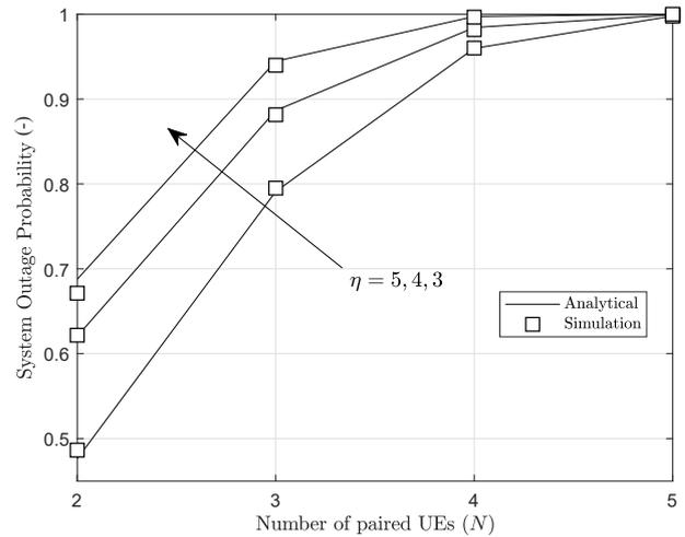
**Fig. 4:** Outage probability versus the number of paired users ( $N$ ) where  $\bar{R}_i = 0.2 \text{ bits}\cdot\text{s}^{-1}\cdot\text{Hz}^{-1}$  and  $\delta_\epsilon = -10 \text{ (dB)}$ .
