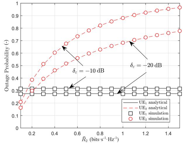
**Fig. 3:** Outage probability at each UE<sub>*i*</sub> with  $N = 2$ ,  $\bar{R}_1 = 0.2 \text{ bits}\cdot\text{s}^{-1}\cdot\text{Hz}^{-1}$  and  $P_1 = 0.9$ .
