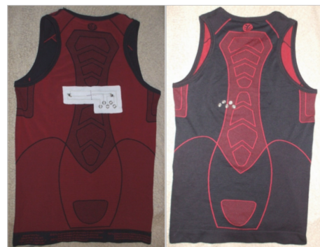
Fig. 5: Proposed intelligent textile with integrated sensors.
