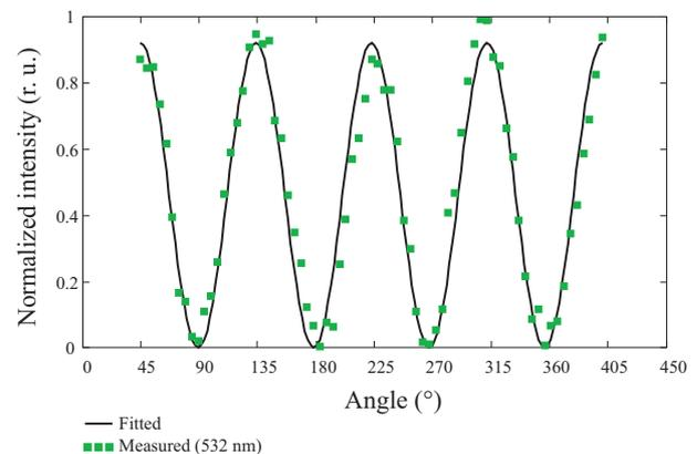
**Fig. 3:** Measured and calculated normalized intensity as function of rotation angle for wavelength  $\lambda = 532$  nm.
