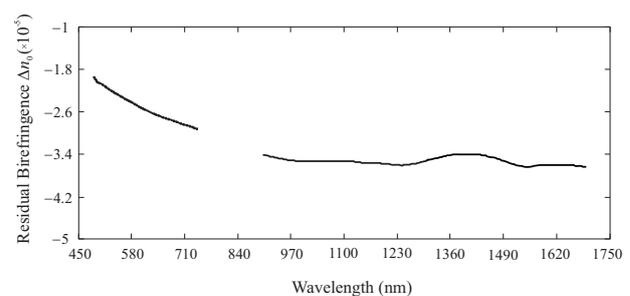
**Fig. 4:** Estimated wavelength dependence of the residual birefringence  $\Delta n_0$  of the investigated PMMA sample.
