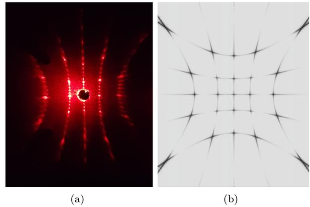
**Fig. 3:** (a) Laue diffraction pattern of 3D PhC woodpile structure with period  $a = 2 \mu\text{m}$ , irradiated by a monochromatic laser light with a wavelength  $\lambda = 635 \text{ nm}$ . (b) Calculated diffraction pattern of woodpile structure with period  $a = 2 \mu\text{m}$ , irradiated by a monochromatic laser light with a wavelength  $\lambda = 633 \text{ nm}$  [11].
