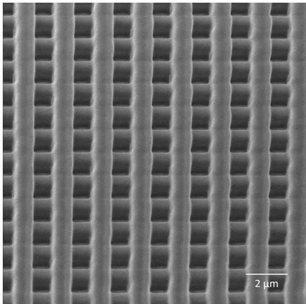
(b) Detail of woodpile structure with well separated dielectric columns by air gaps.
