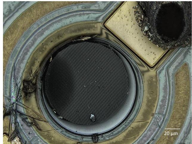
**Fig. 8:** Confocal image of InGaAsN-based photodiode with applied 3D PhC woodpile structure at surface.
