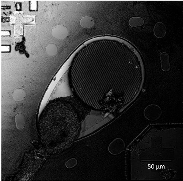
**Fig. 6:** Confocal image of GaAs/AlGaAs based LED with applied 3D PhC woodpile structure at surface.
