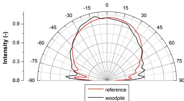
**Fig. 7:** The comparison of reference radiation pattern of clear LED chip and modified LED chip with applied 3D PhC woodpile structure.
