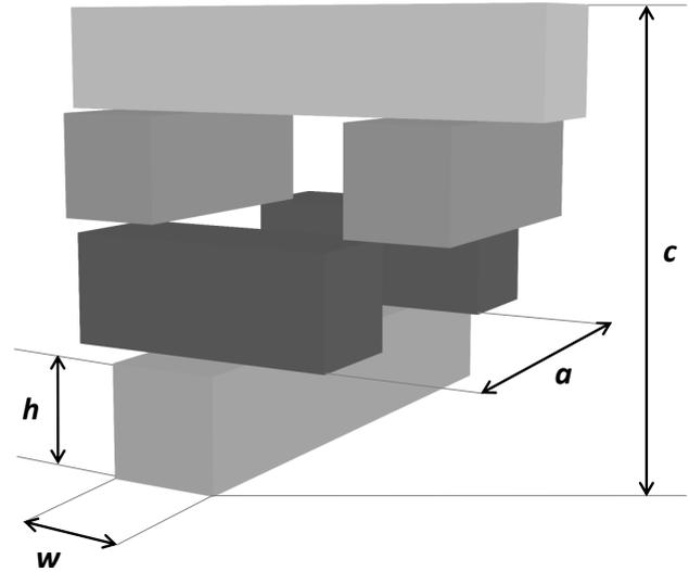
**Fig. 1:** The four-layer sequence arrangement of diamond-like woodpile structure [4].
