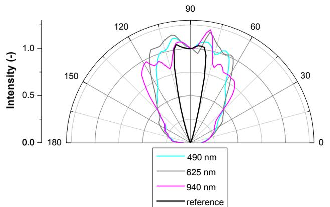
**Fig. 5:**  $\langle 110 \rangle$  cross-section of far-field radiation patterns of modified multi-mode optical fiber by a 3D PhC woodpile structure with period of  $2 \mu\text{m}$  measured at stated wavelengths.
