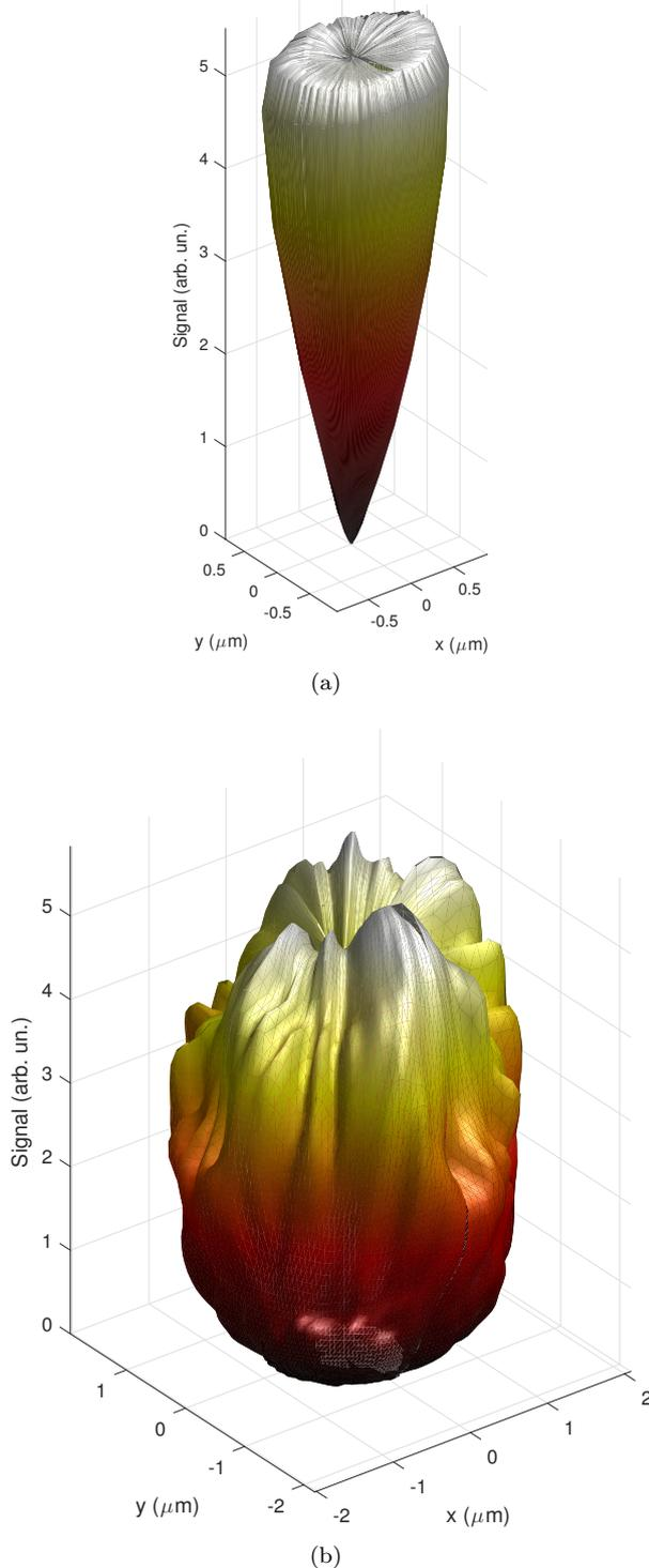
**Fig. 4:** (a) Reference radiation pattern of multi-mode optical fiber with applied smooth cylinder IP-Dip structure measured using LED with a central wavelength of 625 nm. (b) Modified far-field radiation pattern of multi-mode optical fiber with applied 3D PhC woodpile structure measured at wavelength  $\lambda = 625$  nm.
