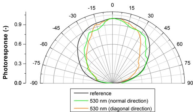
**Fig. 9:** Angular photoresponse of InGaAsN-based photodiode with applied 3D PhC woodpile structure measured in two different directions with respect to the woodpile shown by different colors and compared with reference photodiode.
