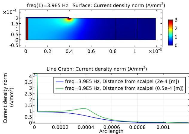
**Fig. 6:** Approximated liver tissue simulation results: current density within the structure (top) and the extraction of the amplitudes of normed current density (bottom).
