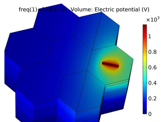
**Fig. 9:** 3D interpretation of electric potential within 3D single part (left) and extended part of liver tissue (right).
