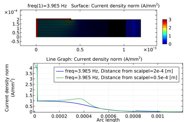
**Fig. 5:** Complex liver tissue simulation results: current density within the structure (top) and the extraction of the amplitudes of normed current density (bottom).
