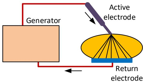
Fig. 1: Principle of configuration for monopolar cutting.
