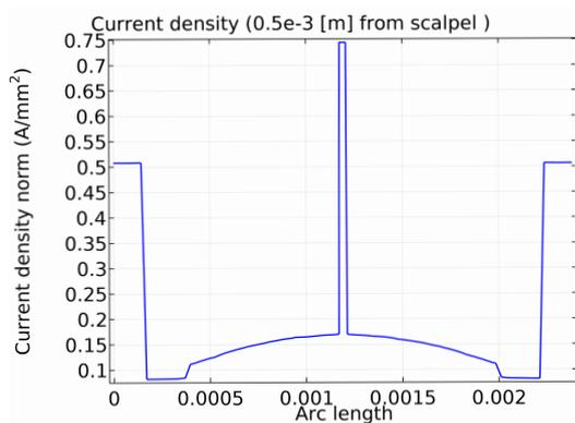
Fig. 11: Current density in slice of the extended part of liver tissue (right).
