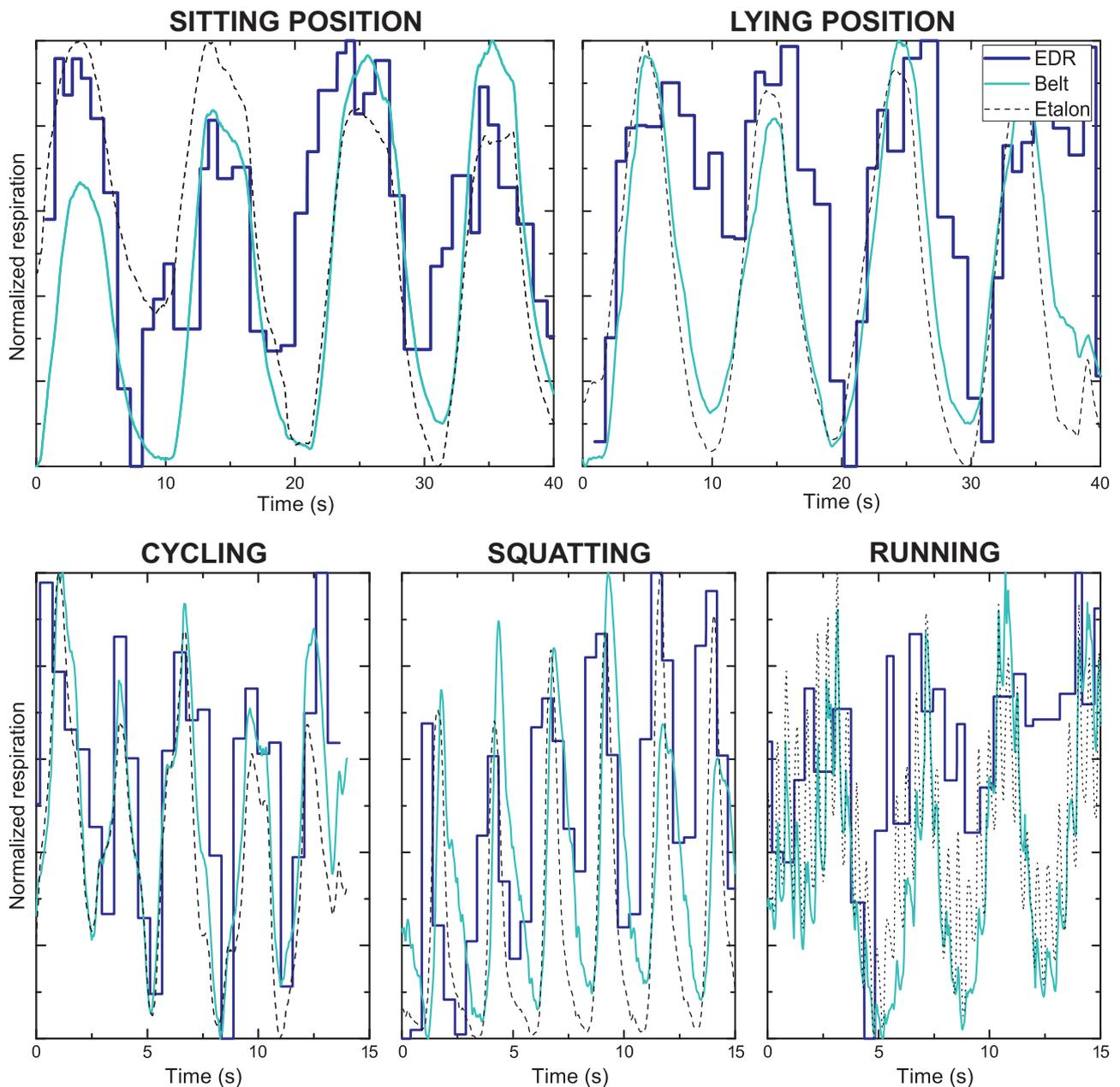
**Fig. 6:** Practical comparison of our EDR system in sensor position  $2.4/135^\circ$  with reference systems measured simultaneously on one proband during 12 hours.
