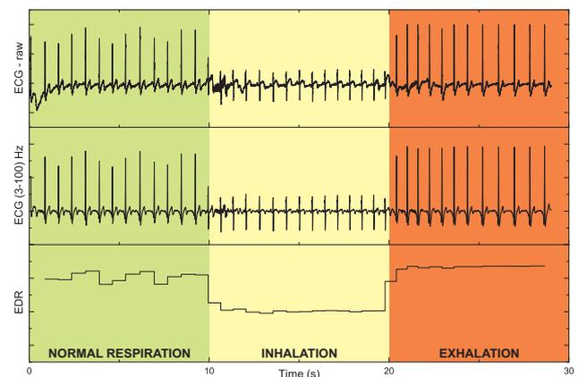
(a) ECG and calculated respiration at position 2.3 and 45° rotation.
