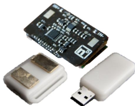
**Fig. 2:** Sensor system (holter). Up - PCB design of sensing unit, Left down - Sensing unit, Right down - Receiver module.
