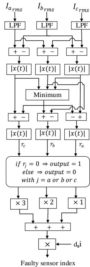
Fig. 6: Isolation scheme of faulty current sensor.
