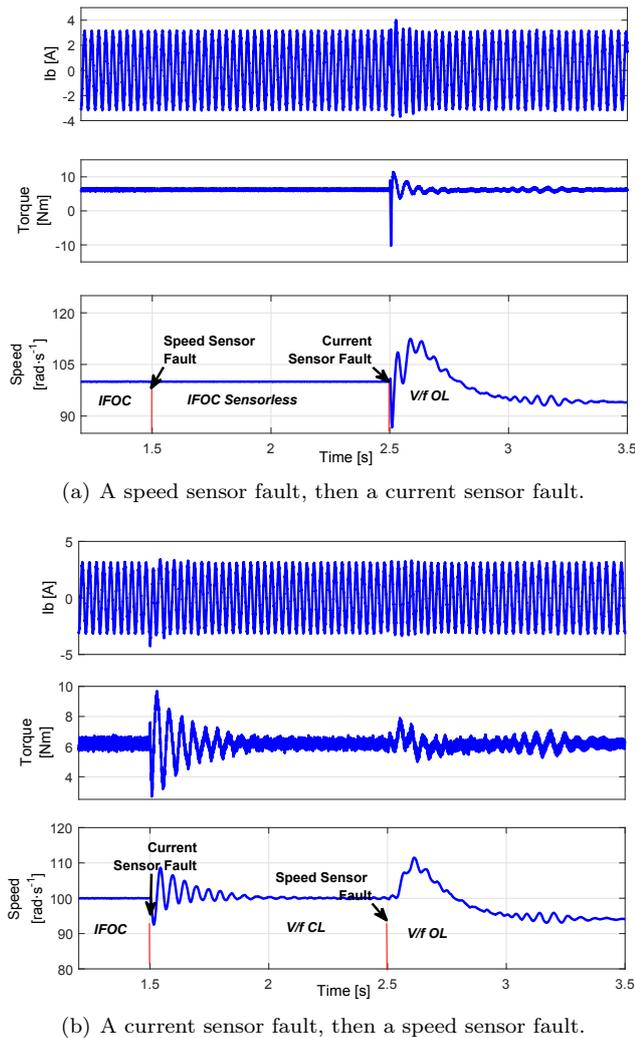
**Fig. 14:** Control reconfiguration due to: (a) a speed sensor fault, then a current sensor fault, (b) a current sensor fault, then a speed sensor fault. With  $\Omega^* = 100 \text{ rad}\cdot\text{s}^{-1}$ ,  $T_l = 6.1 \text{ Nm}$  and  $\phi_r^* = 1 \text{ Wb}$ .
