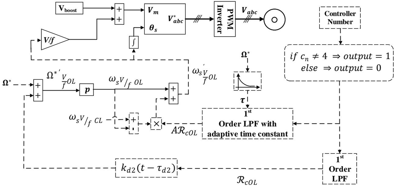
Fig. 13: Modified V/f OL control for soft transition. “Dashed line” stands for all the modifications on the basic scheme.
