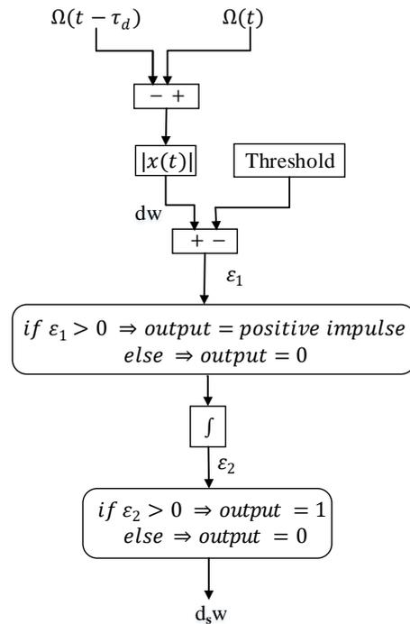
**Fig. 2:** Detection scheme of speed sensor faults. With  $\tau_d = 5 \times T$ .
