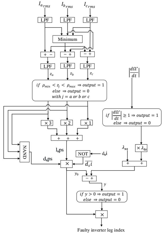
Fig. 8: Faulty leg isolation algorithm.
