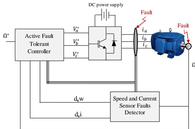
Fig. 10: Overall scheme of the IM drive with AFTC.
