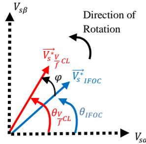
Fig. 11: Reference voltage of IFOC and V/f CL on “ $\alpha\beta$ ” reference frame.
