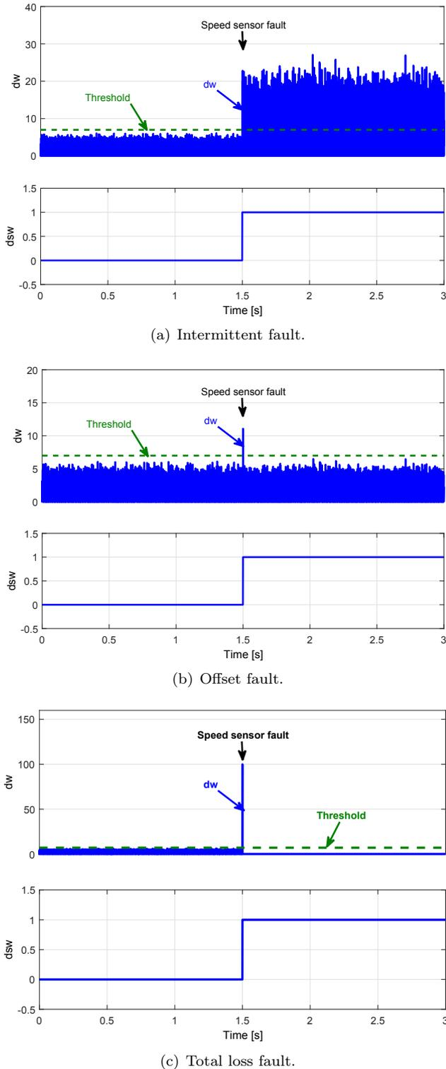
**Fig. 3:** Detection results of speed sensor faults: (a) intermittent fault, (b) offset fault, (c) total loss fault.
