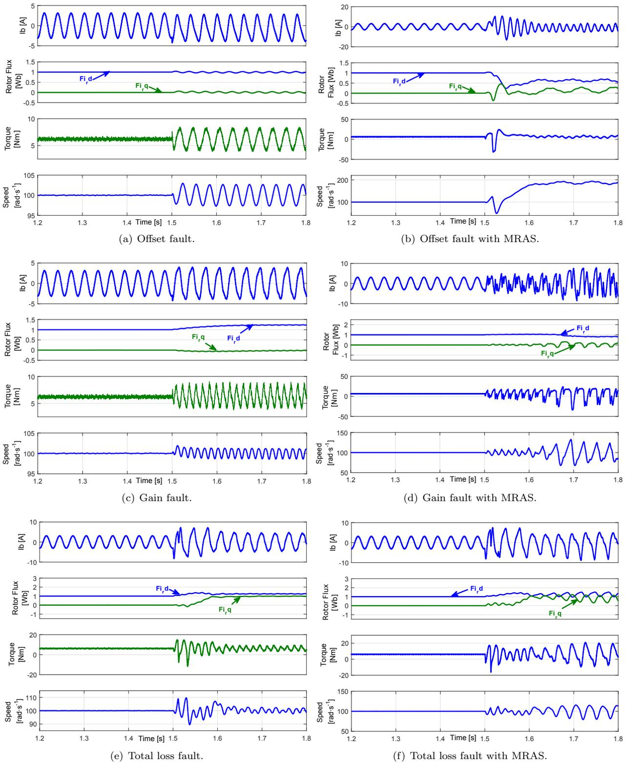
**Fig. 4:** Phase current, rotor fluxes on “dq” reference frame, torque and actual speed in presence of current sensor fault of phase “b” with speed sensor and with MRAS.  $\Omega^* = 100 \text{ rad}\cdot\text{s}^{-1}$ ,  $Tl = 6.1 \text{ Nm}$  and  $\phi_r^* = 1 \text{ Wb}$ . Each fault is applied at  $t = 1.5 \text{ s}$ .
