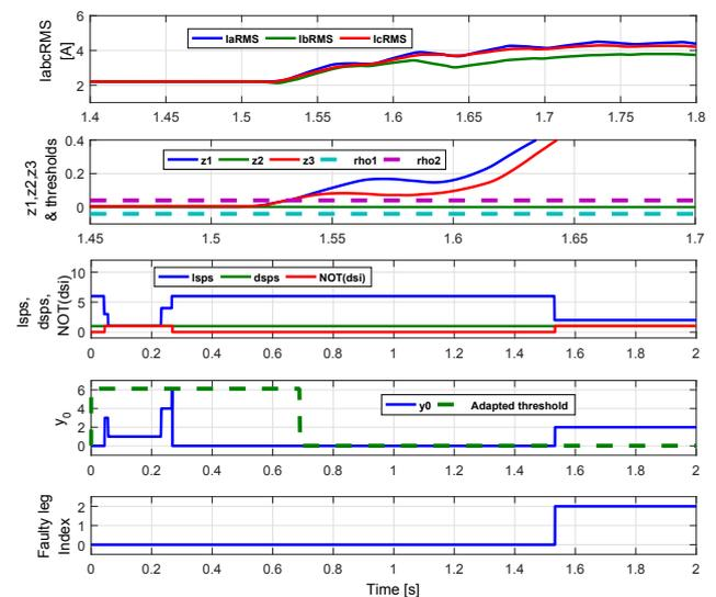
Fig. 9: Faulty leg isolation results.
