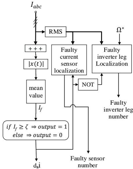
Fig. 5: Global block scheme of current sensor/inverter leg fault detection and isolation.
