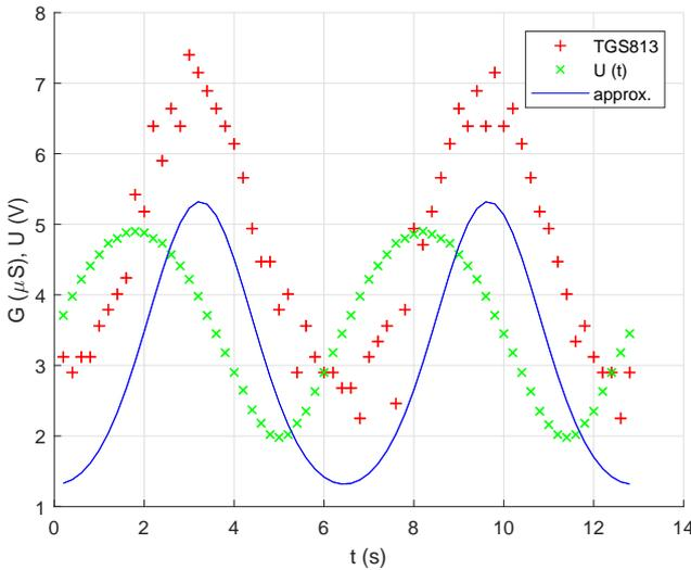
**Fig. 3:** The electrical conductivity  $G(t)$  of the sensor TGS 813 at frequency  $f = 0.156$  Hz in the clean air.  $U(t)$  is the heating voltage.
