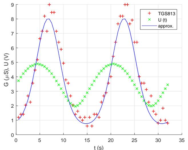
Fig. 2: The electrical conductivity  $G(t)$  of the sensor TGS 813 at frequency  $f = 0.0625$  Hz in the clean air.  $U(t)$  is the heating voltage.
