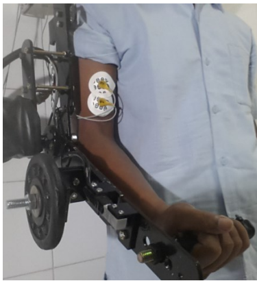
Fig. 1: The Exoskeleton frame to synchronize the elbow-joint motion.
