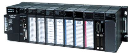
Fig. 5. The view of controller GE FANUC of series 90-30
