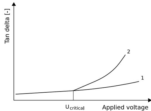
Fig. 2: Dissipation factor versus applied voltage.
