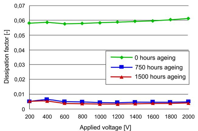
Fig. 6: Dissipation factor of Kraft paper impregnated with a mineral oil.
