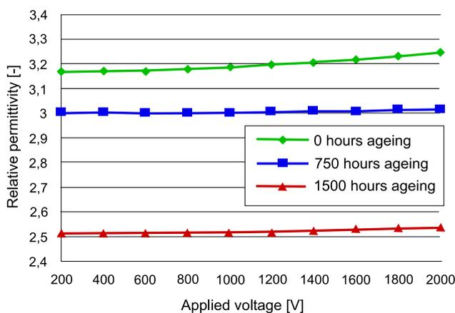
Fig. 4: Relative permittivity of the Kraft paper impregnated with a mineral oil.
