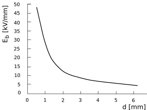
Fig. 1: Dependence of the electrical breakdown strength on the insulation thickness.
