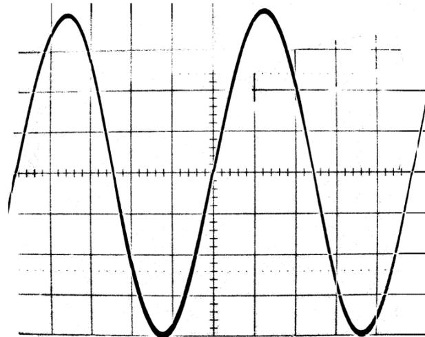
**Fig. 3:** Sine wave generated by MCU (H: 4 ms per div, V: 80 V per div).
