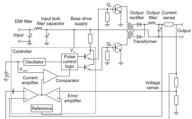
Fig. 1: A walk through a representative switching regulator circuit [12].
