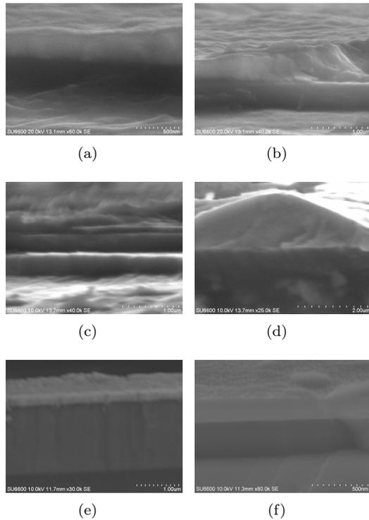
**Fig. 5:** Example SEM images of fractures of annealed Ti/Al/Ni/Au metallization and AlGaIn/GaN heterostructure made at room temperature (a), (b), immediately after bath in LN<sub>2</sub> (c), (d) and fractured during technological process (e), (f).
