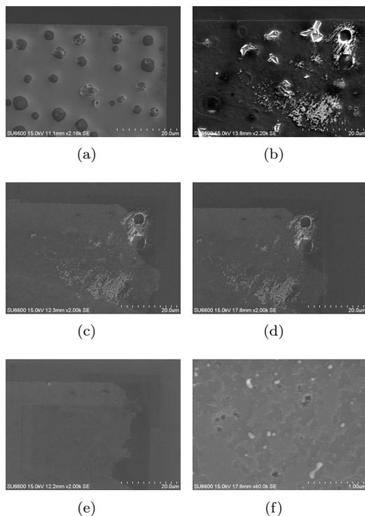
**Fig. 3:** SEM images of metallization surface before etching (a), and remained metallizations layers after etching of (b) Au, (c) Ni, (d) Al, (e) and (f) Ti.
