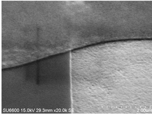
**Fig. 2:** SEM image embracing three types of areas: metallization on etched GaN (A) and mesa (A'), mesa surface (B), etched GaN (C).
