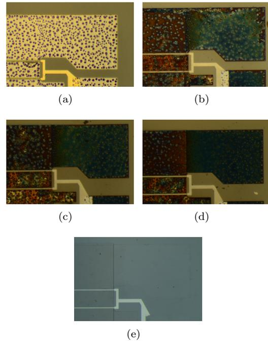
**Fig. 1:** Optical images of metallization surface (a) before etching and after etching of (b) Au, (c) Ni, (d) Al and (e) Ti.
