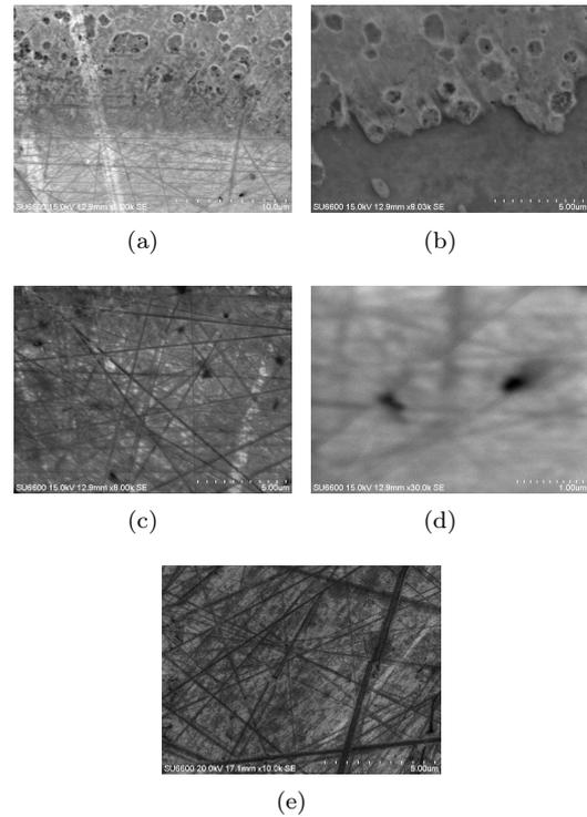
**Fig. 6:** Example SEM images of microsections of annealed Ti/Al/Ni/Au metallization and AlGaIn/GaN heterostructure.
