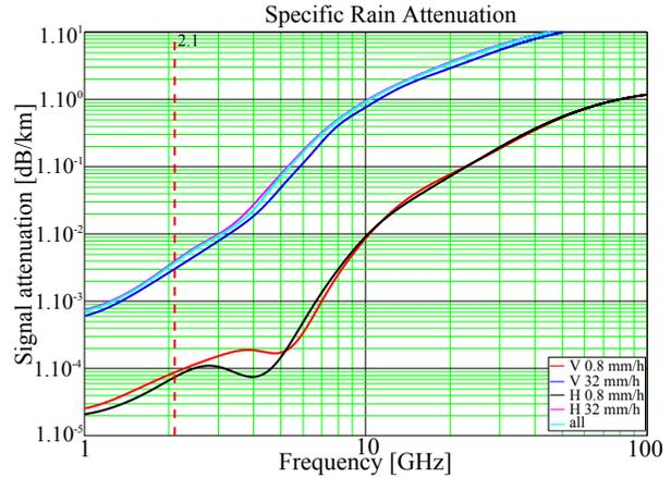
Fig. 2: Graph of the signal attenuation at 0.8 (annual average density) and 32 mm·h<sup>-1</sup> (relative rain rate for 0.01 %).
