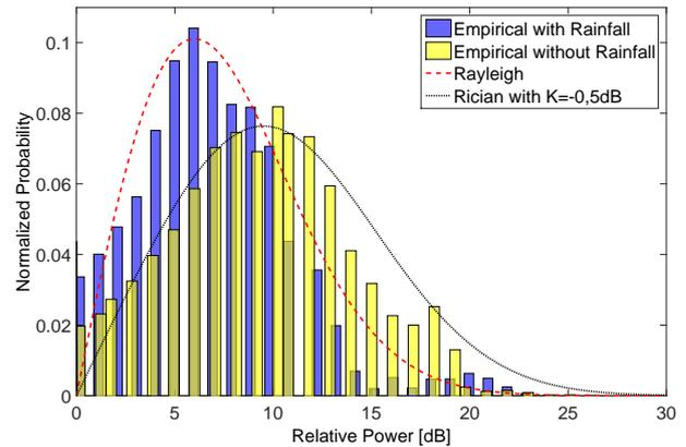
**Fig. 4:** Fitting the probability density functions to the empirical data for NodeB with PSC 444.
