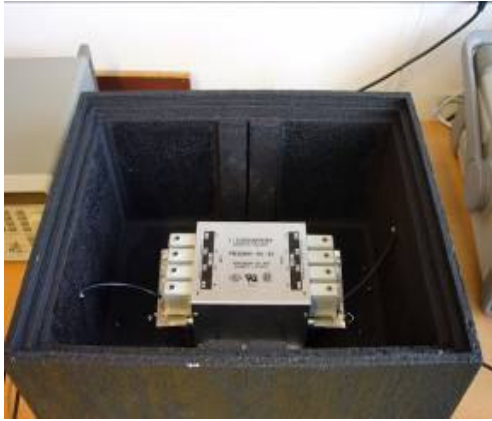
Fig. 7. Measuring chamber with EMC four wire power filter.
