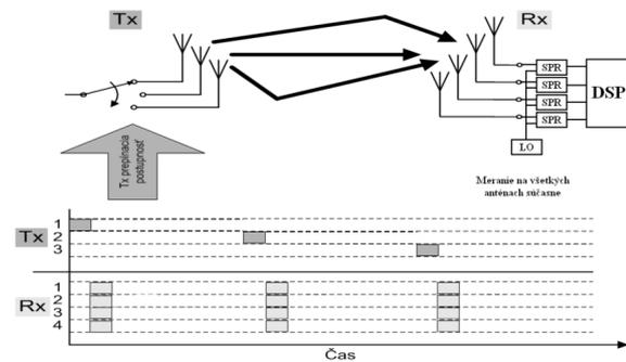
Fig. 3. The principle of MIMO channel sounding
