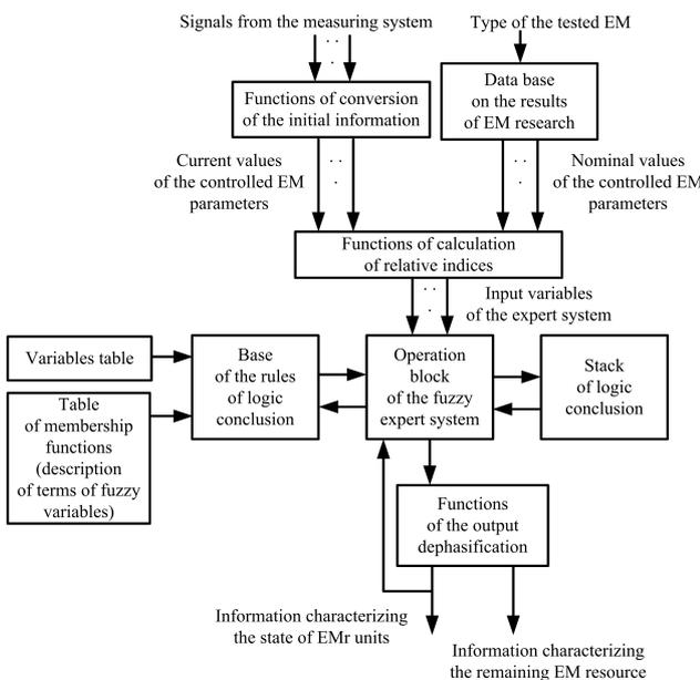
Fig. 1: Diagram of an expert system for estimation of the reliability of EMs with functions of fuzzy conclusion.
