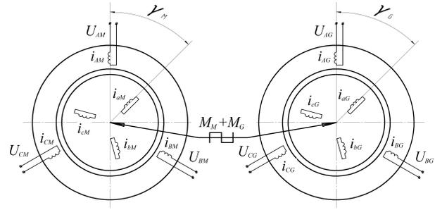
Fig. 1: The system of the engine-generator with a common shaft.
