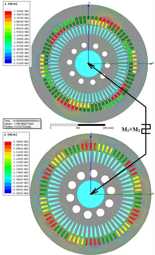
Fig. 6: Interconnected model of electromagnetic fields in the induction motor - asynchronous generator with a common shaft.
