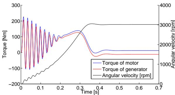
Fig. 3: The electromagnetic torque of the motor and generator, the acceleration curve.
