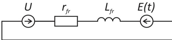
Fig. 5: Equivalent circuit of phase stator.
