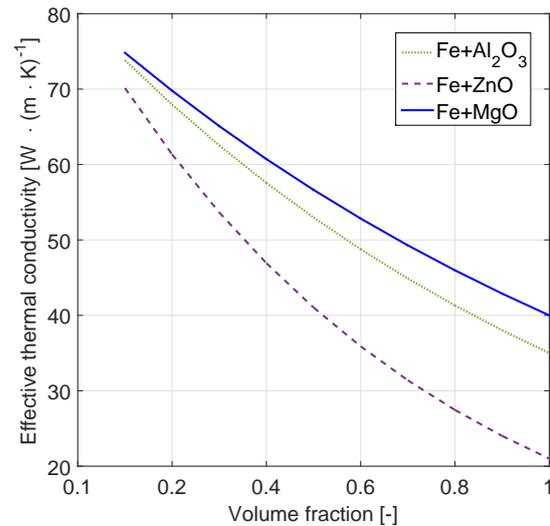
**Fig. 8:** Effective thermal conductivity of TIMs Iron/Oxides nanocomposites with various nanoparticles.
