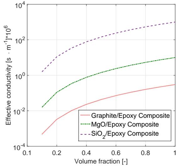
Fig. 5: Effective conductivity of Epoxy Polymeric composites.
