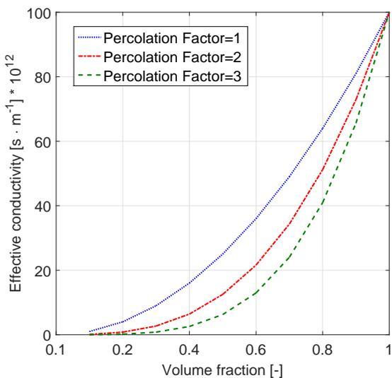
Fig. 4: Effective conductivity of Al<sub>2</sub>O<sub>3</sub>/Epoxy polymeric composites.
