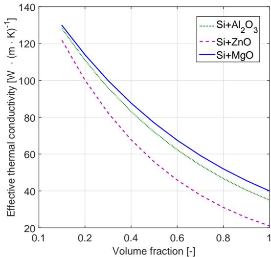
Fig. 10: Effective thermal conductivity of TIMs Silicon/Oxides nanocomposites with various nanoparticles.
