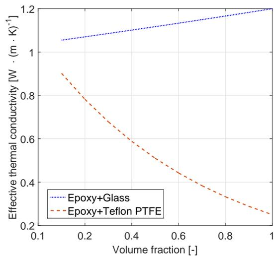
Fig. 13: Effective thermal conductivity of Epoxy/Insulator nanocomposites.
