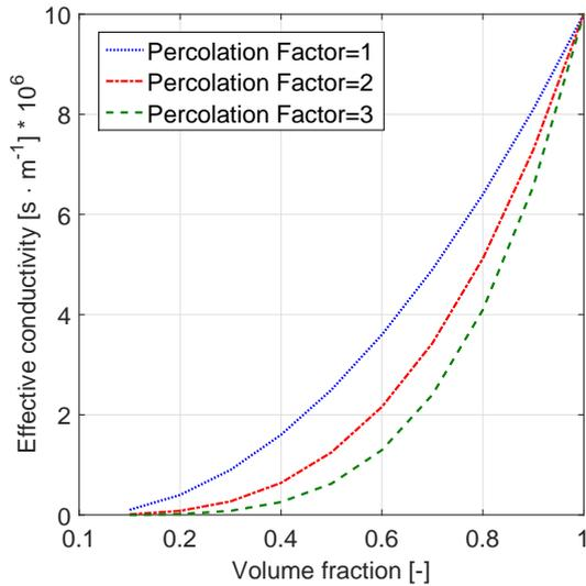
Fig. 3: Effective conductivity of Iron/Epoxy polymeric composites.
