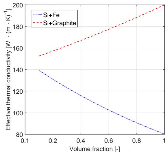
**Fig. 9:** Effective thermal conductivity of TIMs Silicon/Metal nanocomposites with various nanoparticles.
