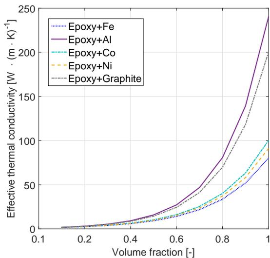
Fig. 11: Effective thermal conductivity of TIMs Epoxy/Metal nanocomposites with various nanoparticles.
