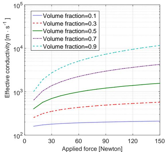
Fig. 6: Effective conductivity of SiO<sub>2</sub>/Epoxy composites.
