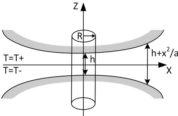
Fig. 2: Schematic diagram for cylindrical region between two spherical particles [26].
