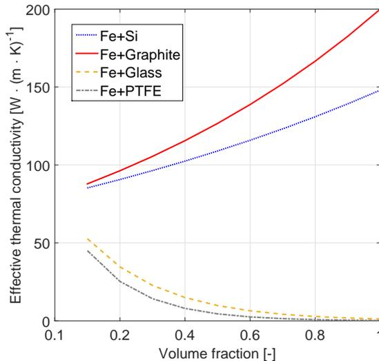
**Fig. 7:** Effective thermal conductivity of TIMs Iron/Polymer nanocomposites with various nanoparticles.
