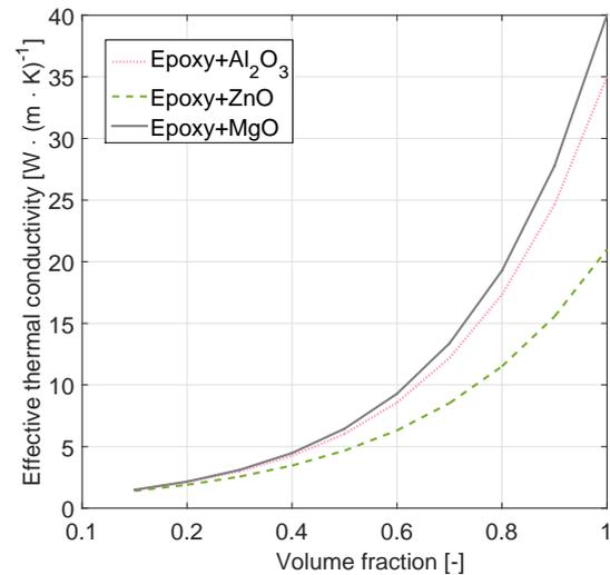
Fig. 12: Effective thermal conductivity of TIMs Epoxy/Oxide nanocomposites with various nanoparticles.
