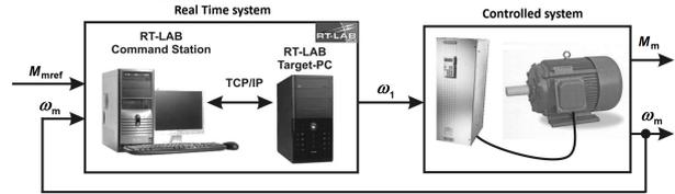
Fig. 11: Layout of the implementation workplace.
