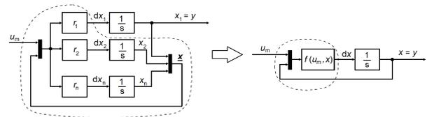
Fig. 2: Procedure of substituting a nonlinear higher order dynamic system by a first order dynamic system.
