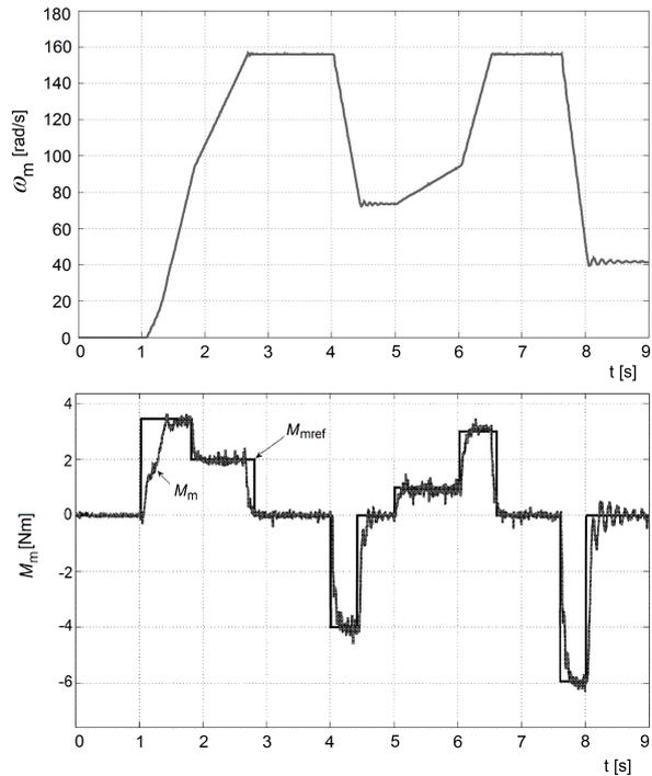
Fig. 12: Measured control responses of angular speed and torque of IM.
