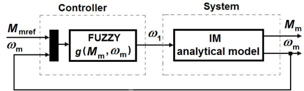
Fig. 8: Control structure based on inverse fuzzy model.
