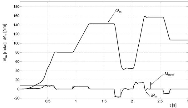
Fig. 10: Properties of control structure based on inverse fuzzy model for various steps of desired torque.
