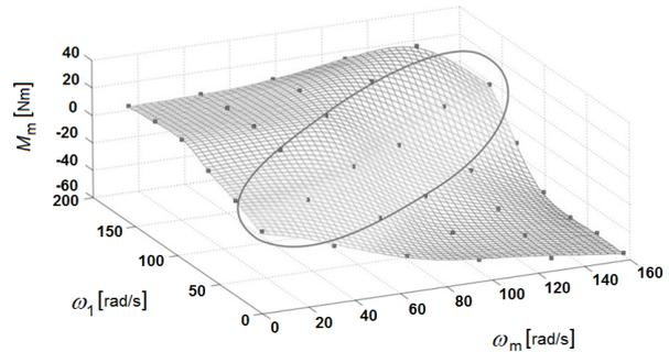
Fig. 6: Characteristic surface of induction motor fuzzy substitute.
