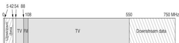
Fig. 3. Frequency band of coax cable [1]
