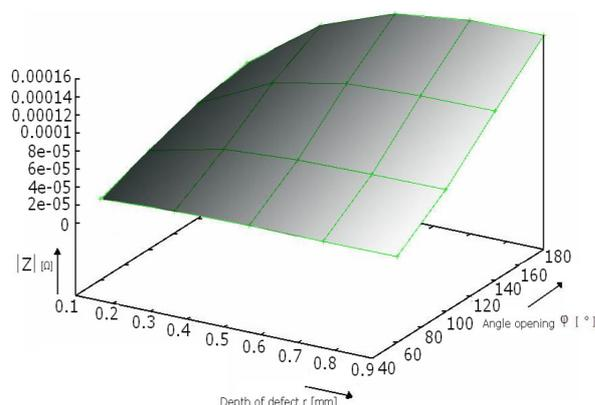
Fig. 10: 3D dimensional dependence of impedance change  $|Z|$  on the depth of defect  $r$  and defect opening angle  $\varphi$
