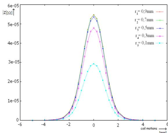
Fig. 9: The simulation result graphics presentation shows a relation of coil impedance change from its movement above the material, where  $\varphi = \langle 40^\circ; 140^\circ \rangle$ , and the defect depth  $r_1=0,9\text{mm}$ ,  $r_2=0,7\text{mm}$ ,  $r_3=0,5\text{mm}$ ,  $r_4=0,3\text{mm}$ ,  $r_5=0,1\text{mm}$
