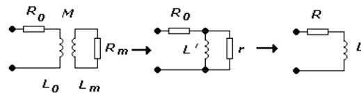
Fig.3: Equivalent circuit of probe on top of object without defect
