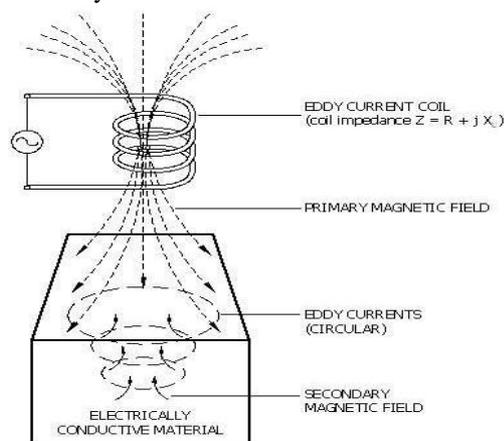
Fig.1: Principle of electromagnetic interaction in ECT
