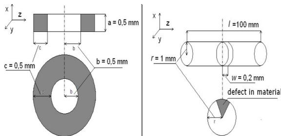
Fig. 7: Dimension of coil and material
